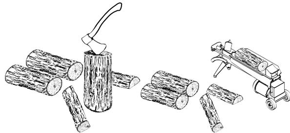
Wood should be split to a range of sizes, from about 3" to 6" (75 mm to 150 mm) in cross section. Having a range of sizes makes starting and rekindling fires much easier. Often, the firewood purchased from commercial suppliers is not split finely enough for convenient stoking. It is sometimes advisable to resplit the wood before stacking to dry.
