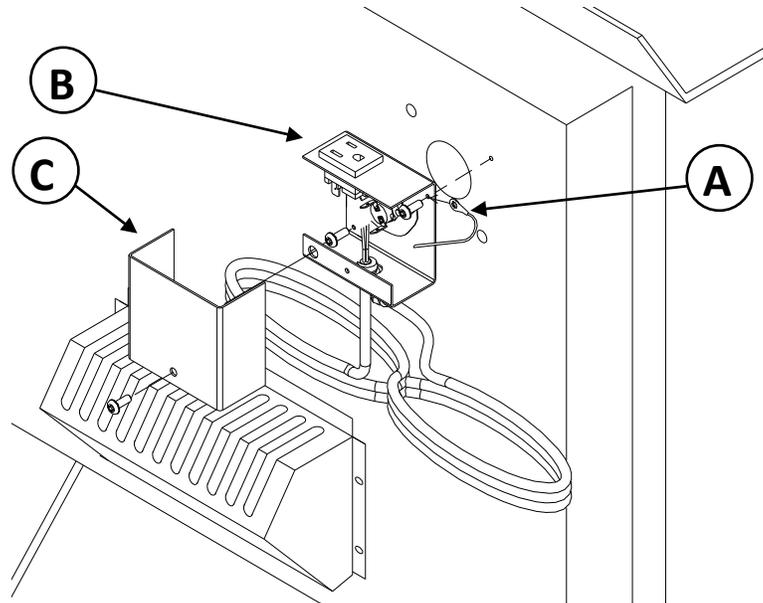
When using the blower without the thermodisc, allow the stove to reach operating temperature (approximately one hour), before turning it on. The increased airflow from the blower cools the firebox and could affect the start-up combustion efficiency if the blower is turned on too early.
