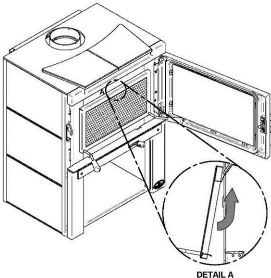
Lean the upper part of the fire screen against the top door opening making sure to insert the top fire screen brackets behind the primary air deflector as in (Detail A).
