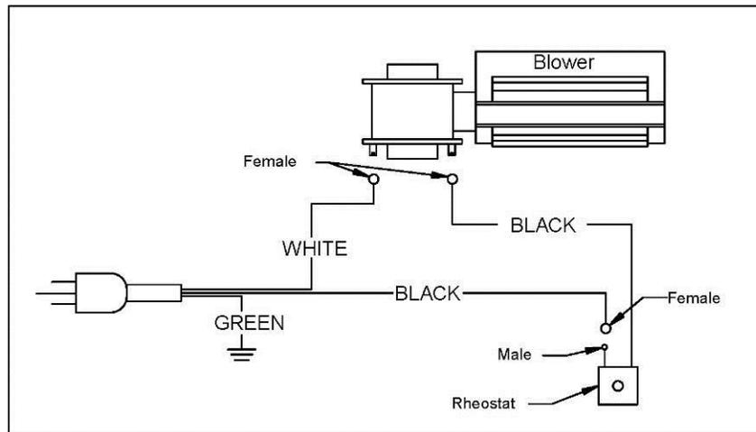
**CAUTION: ENSURE THAT THE BLOWER'S AND/OR THE THERMODISC'S POWER CORD ARE NOT IN CONTACT WITH ANY SURFACE OF THE STOVE TO PREVENT ELECTRICAL SHOCK OR FIRE DAMAGE. DO NOT RUN THE POWER CORD BENEATH THE STOVE.**
