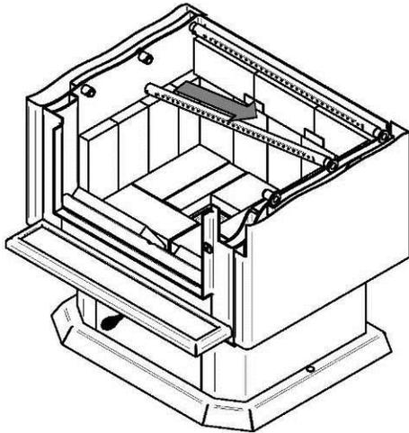
2. Starting with the rear tube, lean and insert the right end of the secondary air tube into the rear right channel hole. Then lift and insert the left end of the tube into the corresponding nozzle in the left channel.
