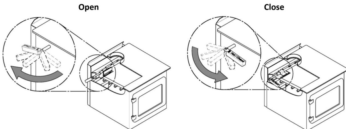
**CAUTION: NEVER LEAVE THE REMOVABLE HANDLE INTO THE SMALL ROD EXTENSION UNLESS YOU ARE BUILDING A FIRE OR RELOADING THE UNIT. THE HANDLE SHOULD BE REMOVED FROM THE STOVE AT ALL OTHER TIMES AND PLACED ON ITS HANDLE SUPPORT (A).**
