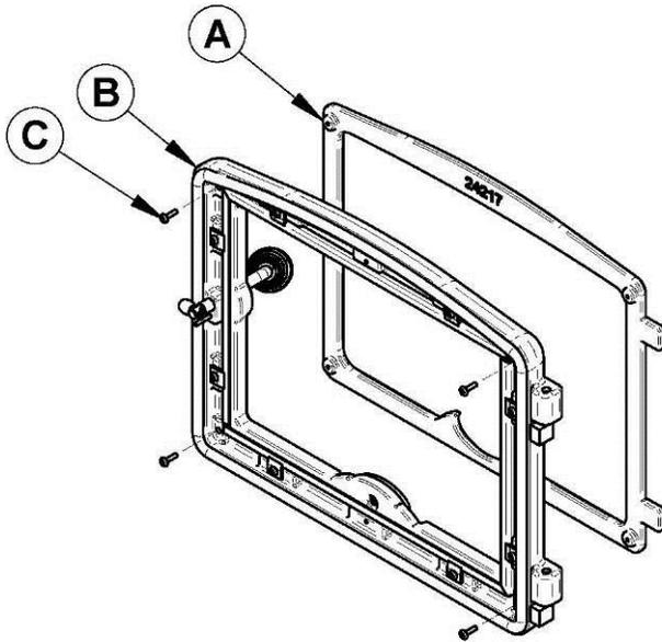
Position the overlay (A) on the door frame (B) and secure it from the inside of the door using the 4 included screws (C).
