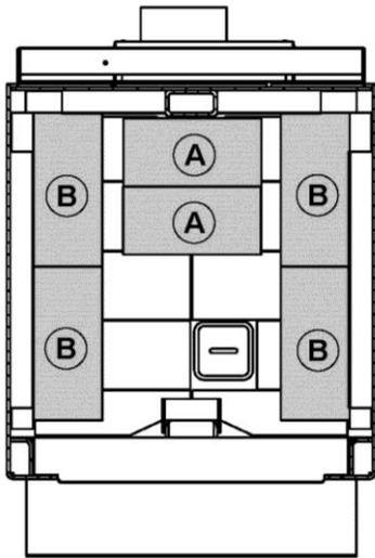
For transportation purpose, the top bricks have been laid on the bottom of the firebox. It is mandatory to install them on the brick supports before you operate the stove. **Failure to install the bricks as describe below may result in stove damage and will void warrantee.**
