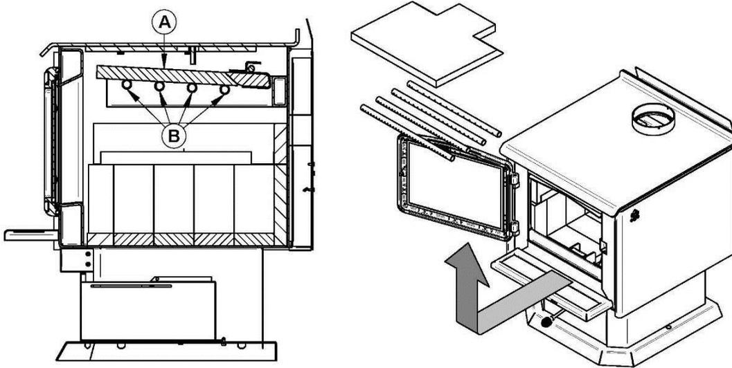
**HOW TO REMOVE AND REPLACE THE BAFFLES OF THE BYPASS DAMPER REGISTRE**
