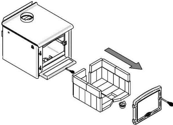
1- Remove the firebricks, the ash dump plug and the loading door from the stove to avoid breaking any parts and facilitate handling in the followings steps.
