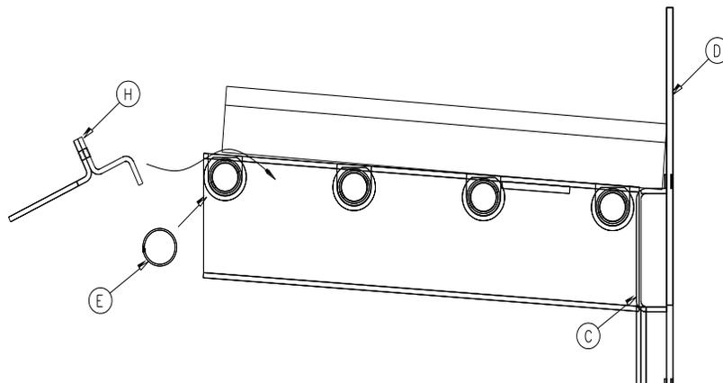
3. Install the middle and rear secondary air tubes ensuring air holes face forward. Install the cotter pins as indicated in the secondary air tubes installation procedure.
