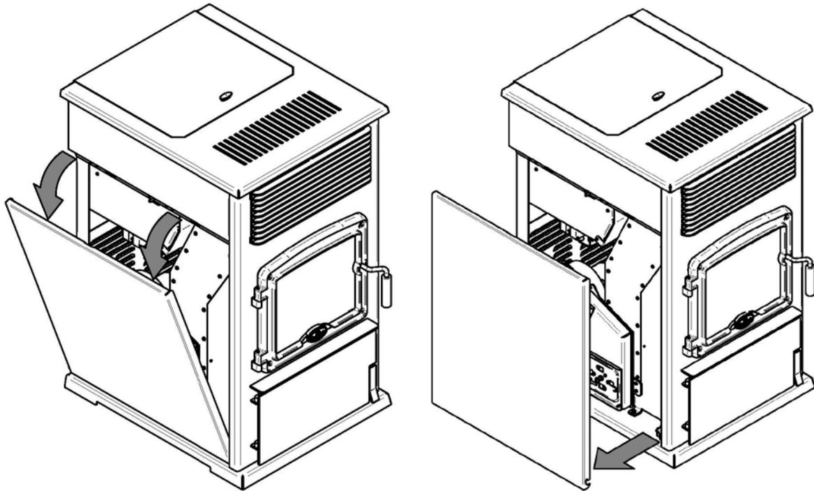
Using a Philips or Robertson screwdriver, remove both clean-out traps by unlocking them. Push the screw and give it a counter-clockwise quarter turn.
