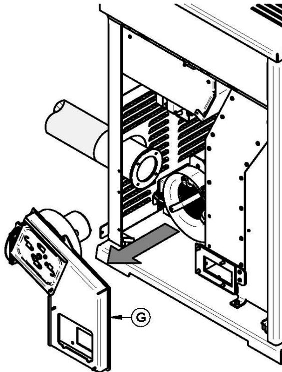
Remove the bolts (H) and nuts (I) to remove the exhaust blower (J)
