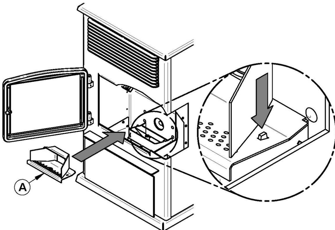
3. If necessary, clean the air intake channel. To reach the air intake channel clean out trap, open the ash drawer access door and remove the ash drawer (A).
