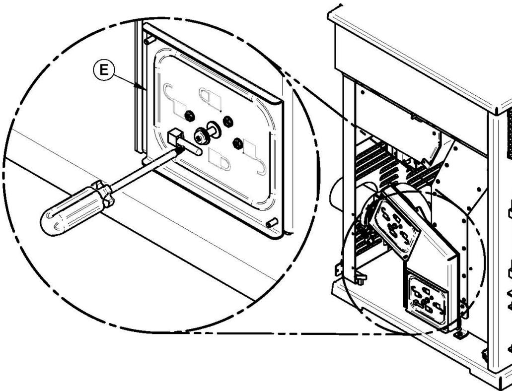
Remove the nuts (F) located in the opening of the trapdoor.
