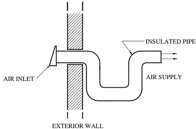
An insulated 3" inside diameter metallic pipe, either flexible or rigid, must be attached to the fresh air intake (D).
