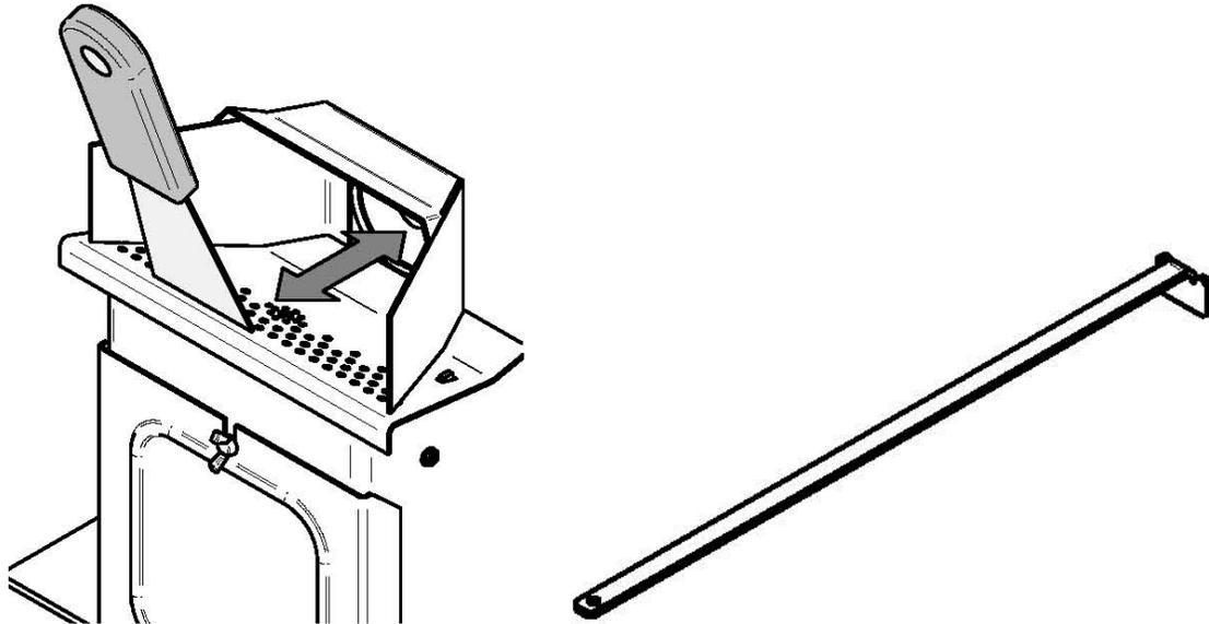
2. The burn pot simply sits onto the air intake channel. You must lift to remove it from the stove. Two small pins guide the burn pot in place. Make sure that the burn pot is well in place before turning on the stove (as shown in the diagram).
