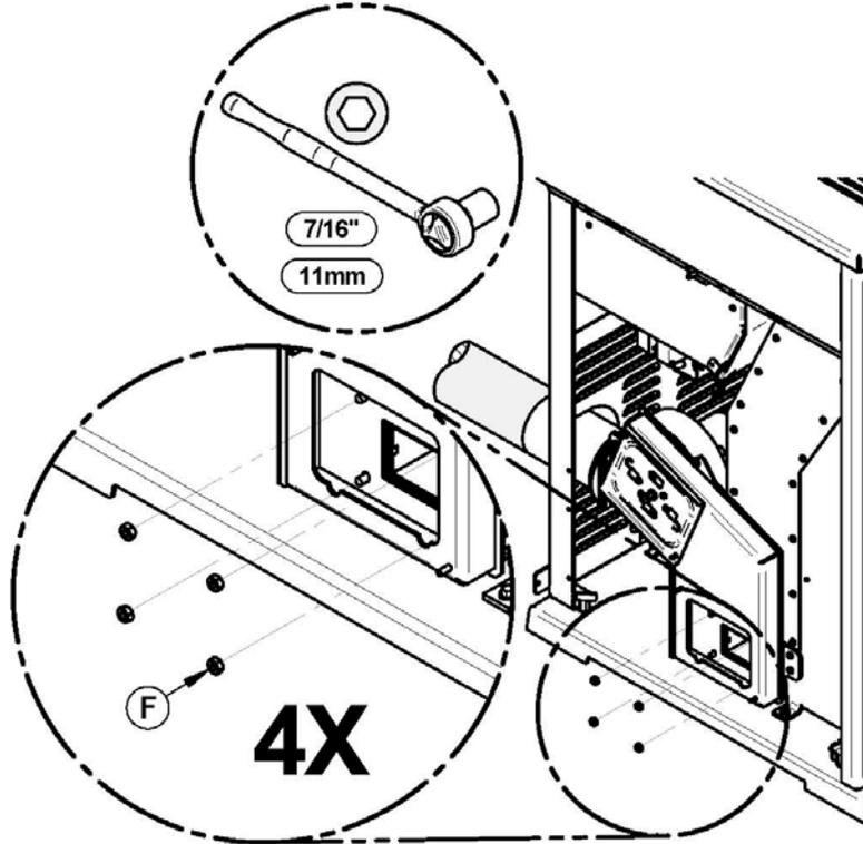
Remove the duct assembly (G).
