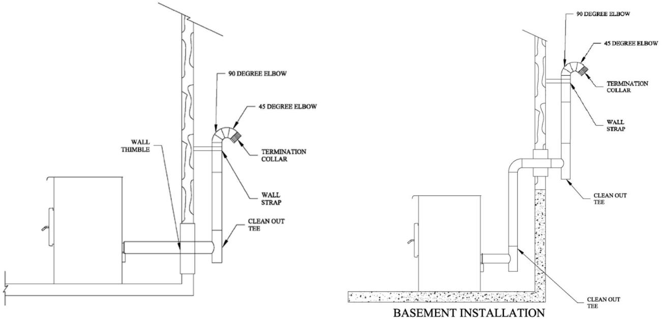
1. Position stove following clearances given in **Section 3, Clearances to Combustible Material** and following vent manufacturer's instructions. Then locate the position of the exhaust pipe in the wall.
