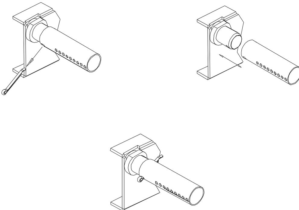
**Figure 4.3 – Secondary Air Tube replacement**
