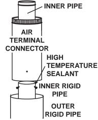
space is tight, we recommend threading the Wolf Steel vent pipe collar or equivalent loosely onto the air terminal connector / vent pipe assembly as it is passed through the attic. The air terminal connector must be located vertically and plumb.
