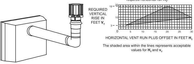
For vent configurations requiring more than one 90° elbow, the following formulas apply:
