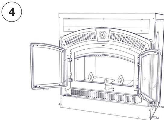
Press bypass rod downwards then inwards to lock into place.
