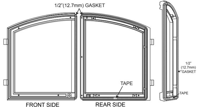
When you return to the other end of the gasket wrap a piece of tape around the other end of the gasket and cut through the center, refer to Figures 1 and 2.
