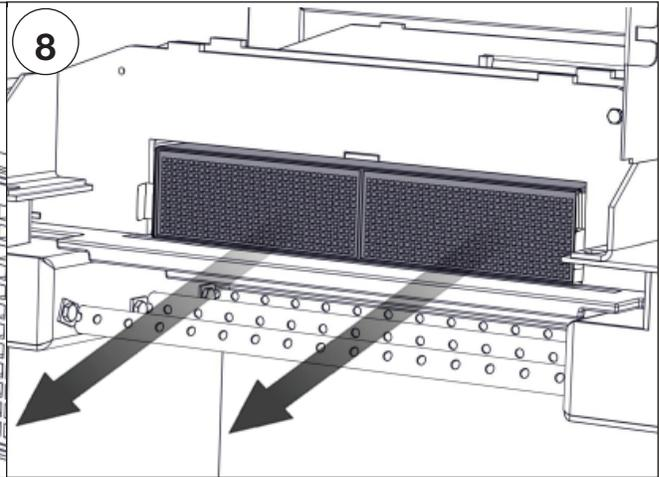
Slide the catalyst forward and out. The steel tabs are friction held and will separate from the catalyst when pulled out.
