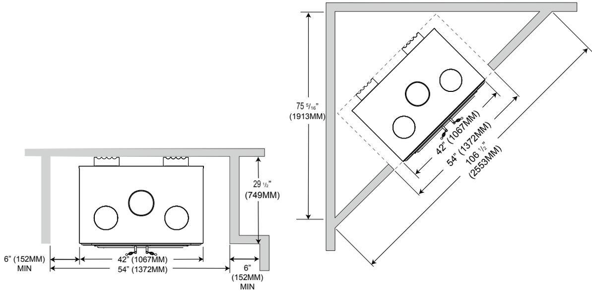
A minimum of 6" (62mm) is required to combustibles from the side of the appliance.
