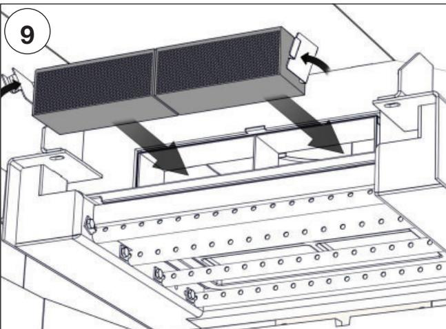
Holding the steel tabs located on either side of the catalyst, slide the new catalyst into the cavity.
