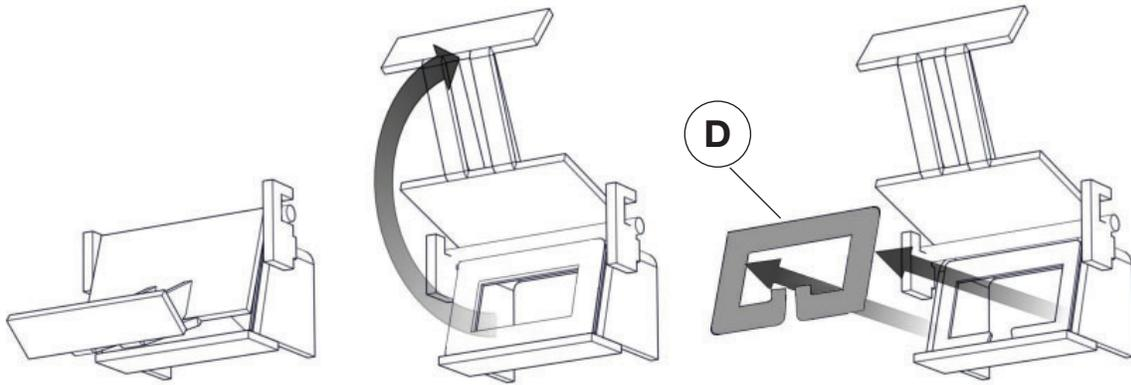
Open dilution door and remove gasket.
