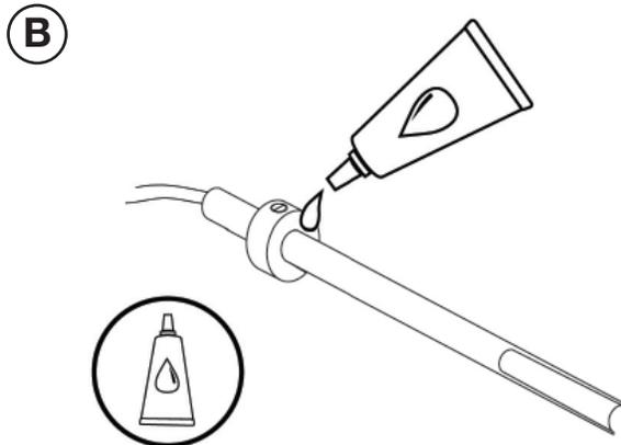
Liberaly spread stove cement (not supplied) along the bottom of depth gauge.
