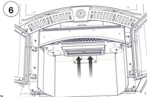
Reach in through the opening of the bypass door to access fasteners.
