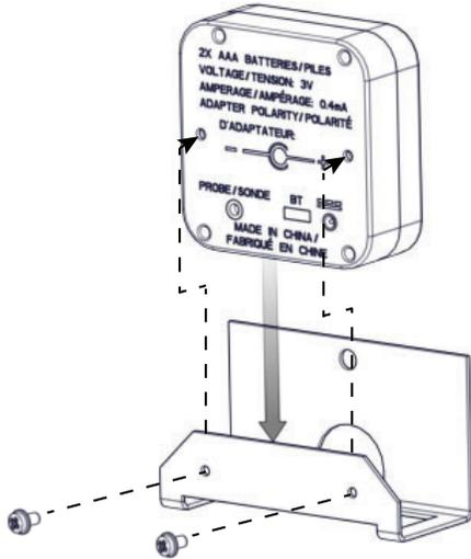
Slide the catalyst temperature monitor into the bracket and attach with screws (supplied).
