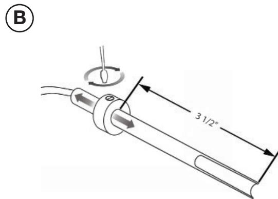
Set the depth to 3.5" and secure with set screw.
