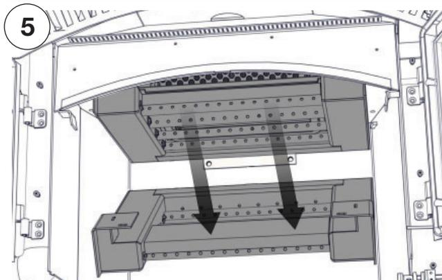
Slide secondary air manifold downward and out to remove. Scrape off gasket from rear and clean surface. Secure new gasket with high temperature silicone (not supplied).
