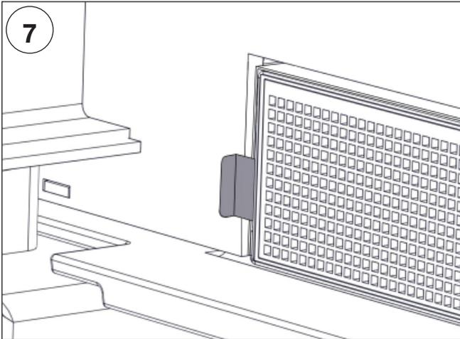
Grab the steel tabs located on either side of the catalyst.
