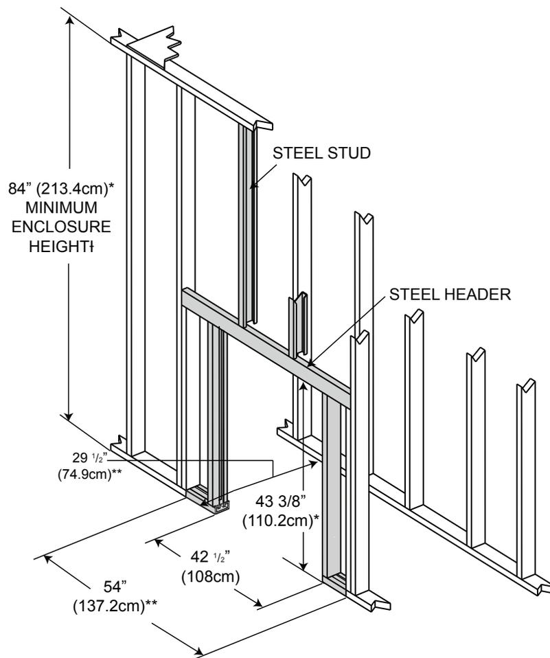
\* Allow for finished floor and hearth thickness when setting these dimensions.
