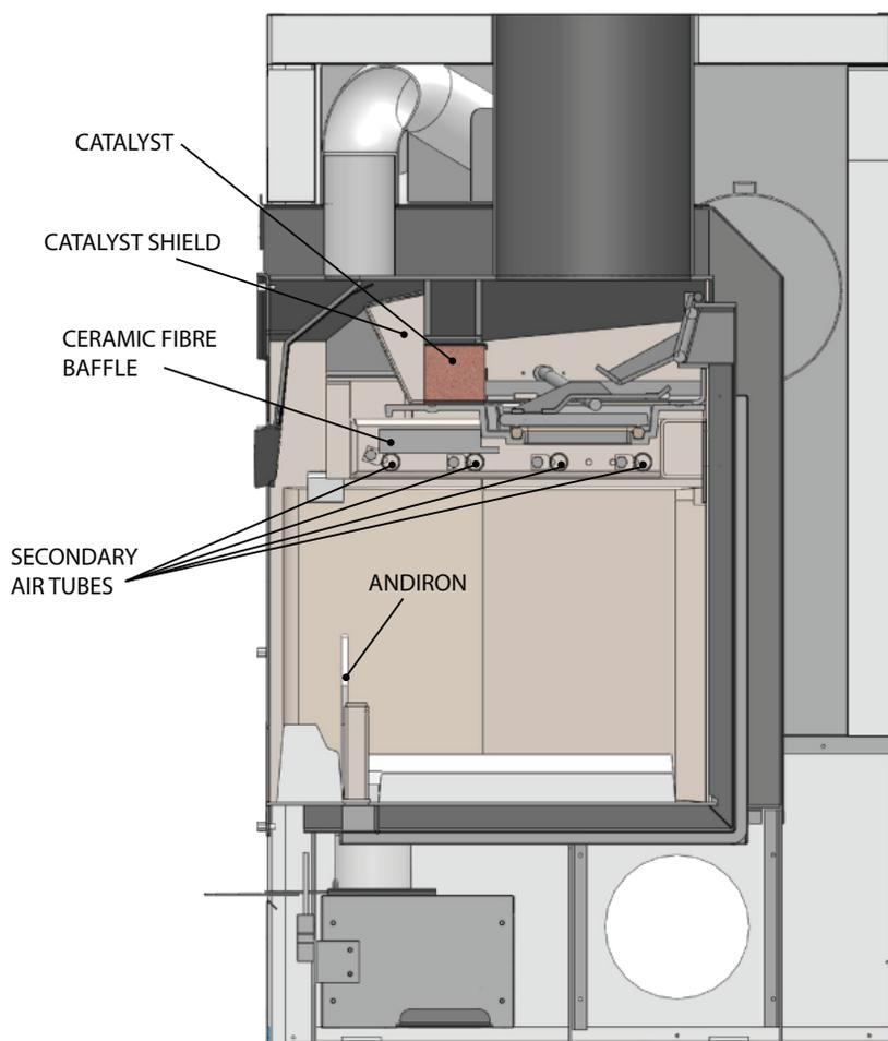
The NZ3000H contains a ceramic fibre baffle, catalyst and catalyst shield. It is important that each of these components are installed correctly prior to operating the appliance.
