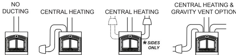
\* When installed with a masonry chimney, the hot air gravity and central heating system can only be installed off the sides.
