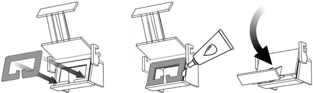
Apply new gasket using stove cement (not supplied) to secure. This is to prevent the ends from fraying and locking the gasket into position of the gasket groove.
