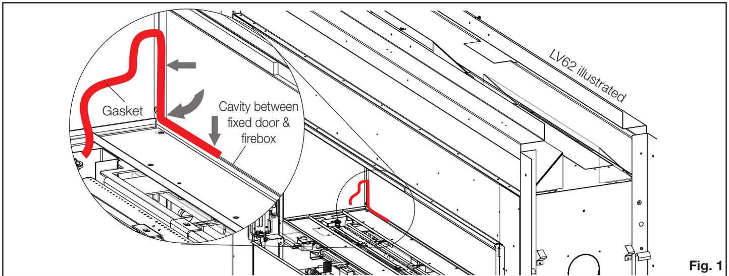
7. Continue working the gasket into the cavity, ensuring it covers the entire distance along the fixed door (**Fig. 2**).
