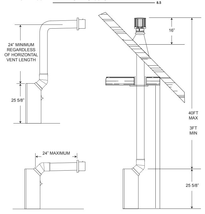
The maximum horizontal run with a 57" vertical rise immediately above the appliance is 20 feet.
