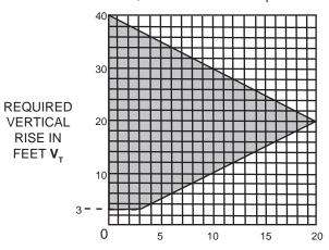
HORIZONTAL VENT RUN PLUS OFFSET IN FEET  $\mathbf{H_T}$  The shaded area within the lines represents acceptable values for  $\mathbf{H_T}$  and  $\mathbf{V_T}$
