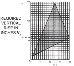
HORIZONTAL VENT RUN PLUS OFFSET IN FEET **H**<sub>T</sub>
