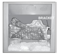
A. Place the rear log, as shown, onto the rear log support brackets. Ensure the cutout on the left underside of the log, fits over the pilot assembly. Bend the bracket on the right side to help retain the rear log.
