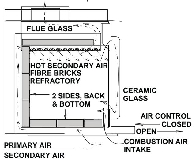
Be sure to provide sufficient combustion air. There are many other appliances in your home competing for air such as: a kitchen range hood, forced air heating devices or a bathroom exhaust fan.
