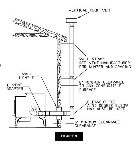
Locate terminations: a) not less than 3 feet above any forced air inlet located within 10 feet; b) not less than 4 feet below or horizontally from, or one foot above, any door, window or gravity air inlet into any building; c) not less than two feet from an adjacent building and not less than 7 feet above grade when located adjacent to a public walkway. Mobile home installations must use a spark arrester.
