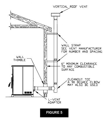
Locate terminations: a) not less then 3 feet above any forced air inlet located within 10 feet; b) not less than 4 feet below or horizontally from, or one foot above, any door, window or gravity air inlet into any building; c) not less than two feet from an adjacent building and not less than 7 feet above grade when located adjacent to a public walkway. Mobile home installations must use a spark arrester.
