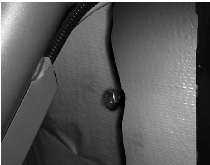
Incorrect Burn: bolt is too far out. (Fig. 3)
