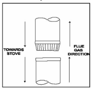
For venting vertically into a Class A chimney, single wall black steel pipe (at least 24 gauge and 6" in diameter) must be used in the room where the stove is installed. Refer to the manufacturer's instructions for the connection to the listed chimney.
