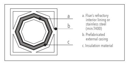
**INSULATION**: flue draught pressure also depends on the difference in the temperature of the hot flue gases and that of the air outside.
