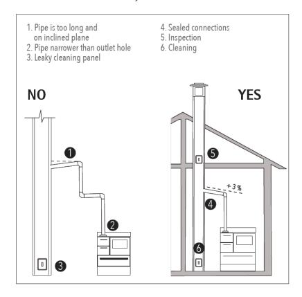
Connecting pipes must be perfectly sealed to each other and to the stove and flue pipe. These precautions must be taken:
