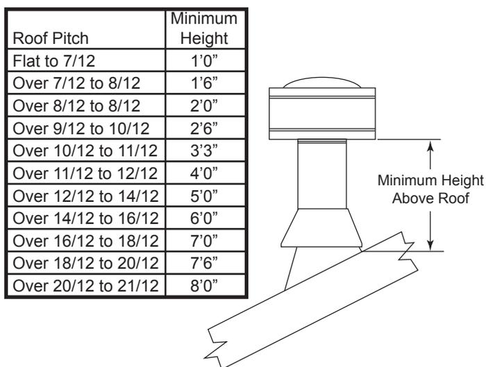
Fig. 44 Minimum Height Above Roof Requirements
