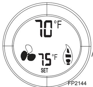
Fig. 62 Thermostatic mode.
