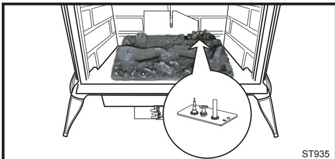
**Fig. 76** Pilot assembly location.
