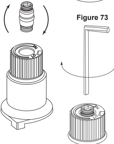
**WARNING:** Do not overtighten the screw. Recommended to grip the wrench by the short side.
