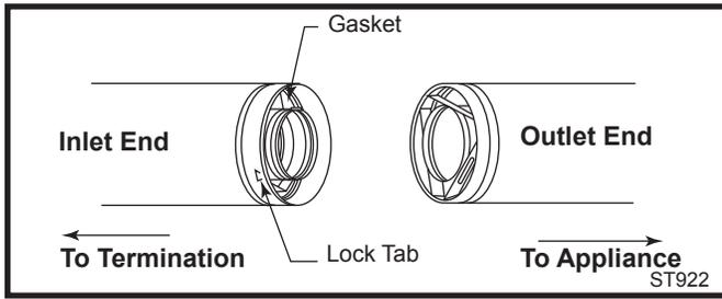
Fig. 33 Joint connection.
