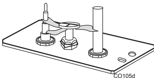
Fig. 56 Correct pilot and burner flame patterns.
