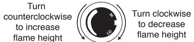
Fig. 55 Flame adjustment knob for SIT valve.
