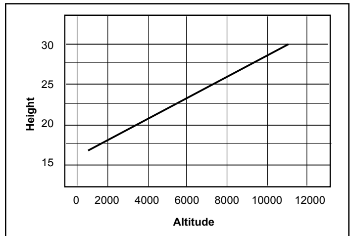
Fig. 2 - Chimney height requirements with 6" chimney and/or chimney connector.
