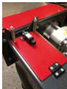
Spring loaded lid with an electrical switch, which stops the delivery auger in case of fuel piling up
