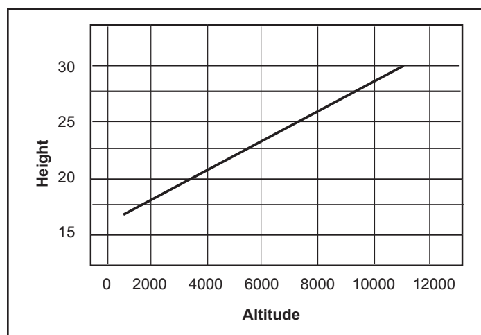
Figure 2 - Chimney height requirements with 6" chimney and/or chimney connector.
