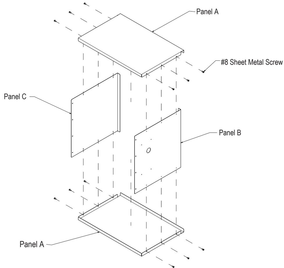
4. Position the assembled filter box on rear of furnace, supporting it firmly up to electrical enclosure, covering the rear distribution blower. Make sure the filter box is tightly pressed to the back of the furnace. Use 4 1/4" bolts (included) to firmly attach the filter box to sides of furnace.
