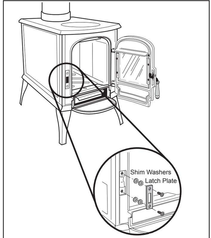
**Figure 9.2** - Remove shim washers to tighten latch engagement.
