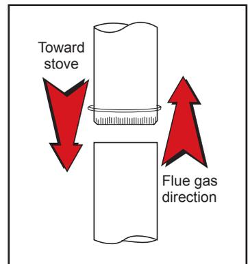
**Figure 5.3** - Chimney connector.
