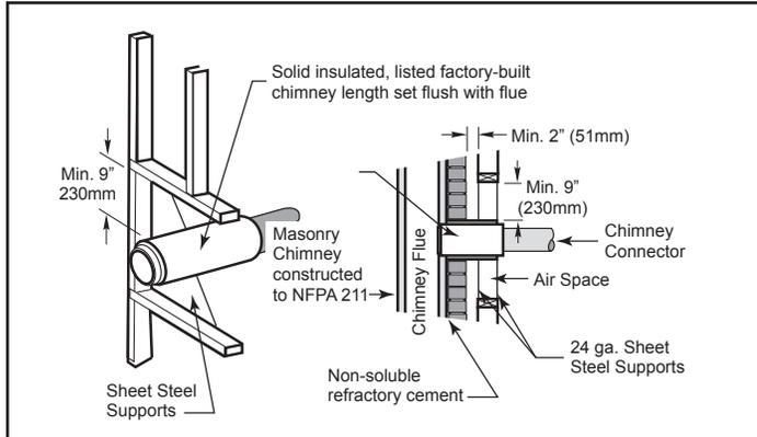
**Figure 5.7 - Wall Pass-through using factory-built insulated chimney section.**
