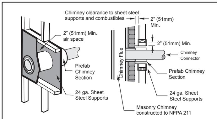
**Figure 5.9 - Wall Pass-through with ventilated steel thimble.**
