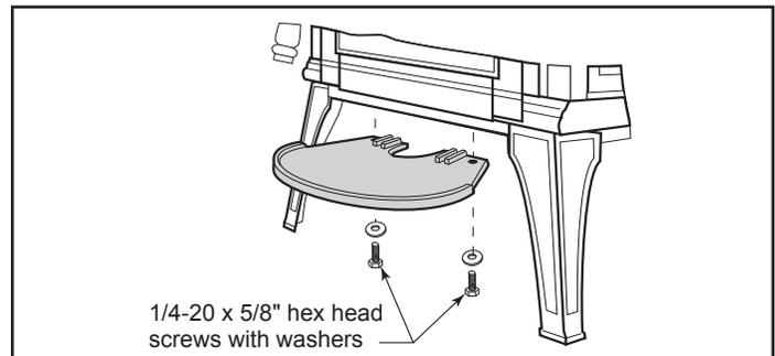
Figure 7.2 - Attach the Ashlip to the bottom plate.
