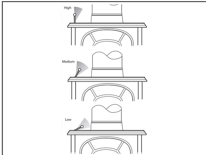
Figure 8.1 - Air inlet shutter settings; Low - Medium - High.
