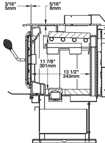
Combustion chamber - side view
