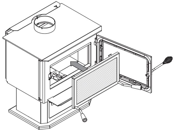
3. Lean the upper part of the fire screen against the top door opening making sure to shove the top fire screen brackets behind the primary air deflector.
