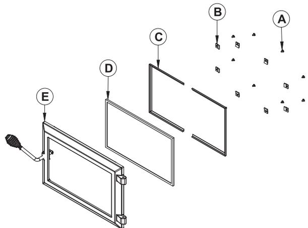
*The two main causes of broken door glass are uneven placement in the door and over-tightening the retaining screws.*
