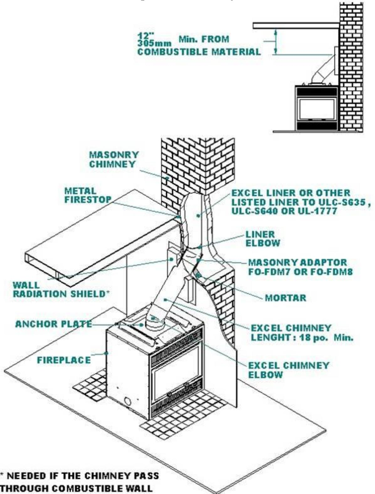
Figure #7: Straight Chimney Installation
