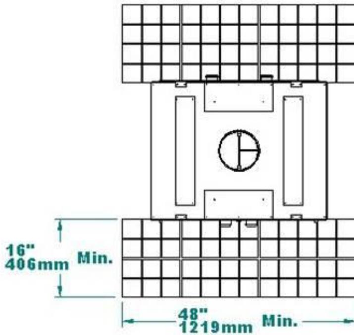
**TOP OF THE NON COMBUSTIBLE SURFACE MUST NOT EXCEED THE BOTTOM OF THE FIREPLACE**
