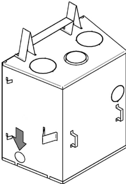
The fresh air intake kit must be installed on the right side of the fireplace.
