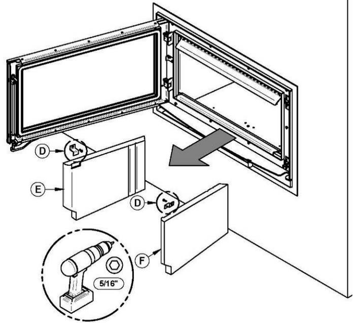
Remove the rear refractory slab (G).
