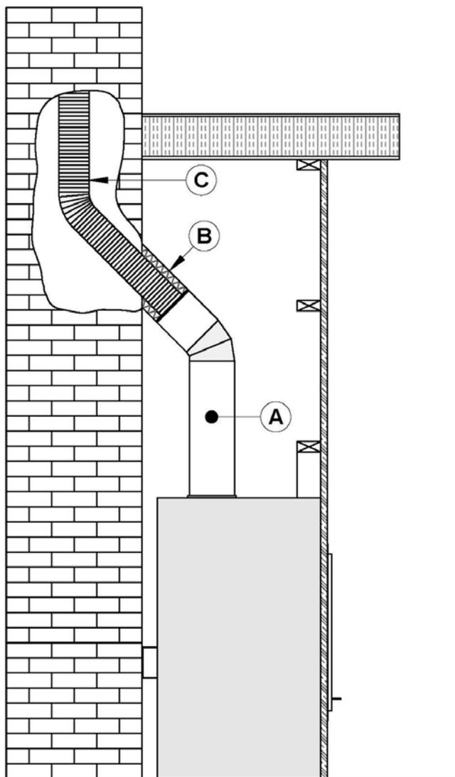
**Note:** Make sure the liner exceeds at least 12" (30 cm) the top of masonry chimney.
