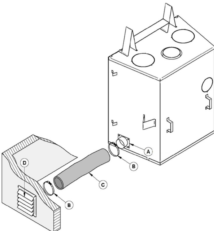
Then, install the flexible pipe\* **(C)** (not supplied) to the fresh air intake adapter **(A)** using one of the adjustable pipe clamps **(B)**. Secure the other end of the pipe to the outside wall termination **(D)** using the second adjustable pipe clamp **(B)**. The outside wall termination **(E)** must be installed outside of the building.
