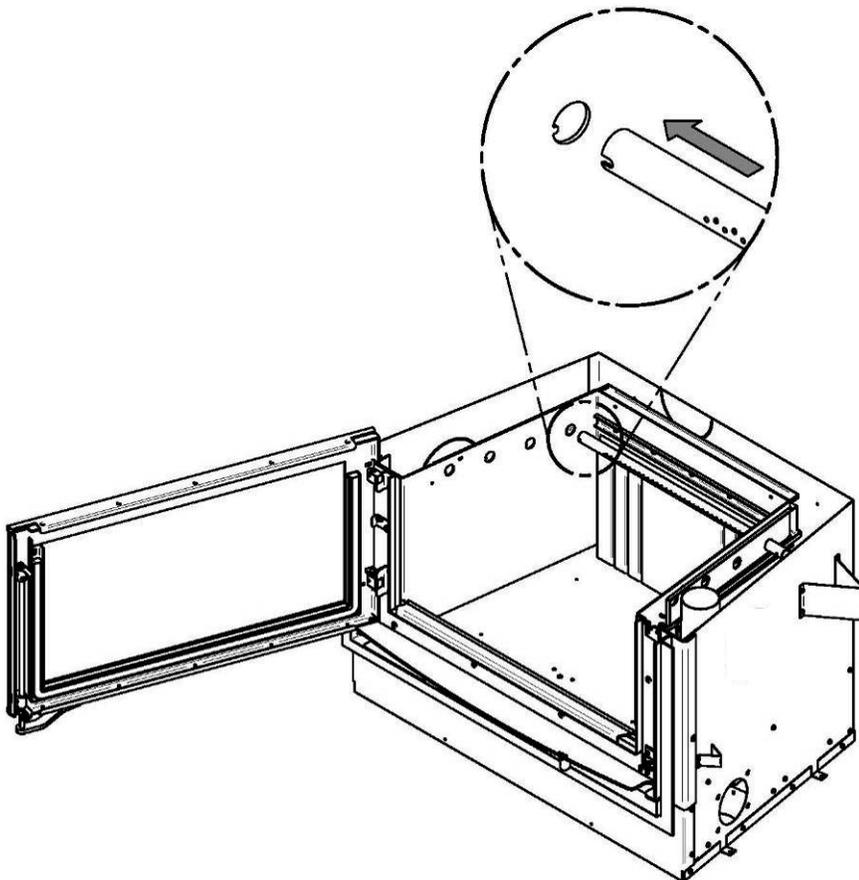
Align the notch in the left end of the tube with the tab of the left air channel hole.
