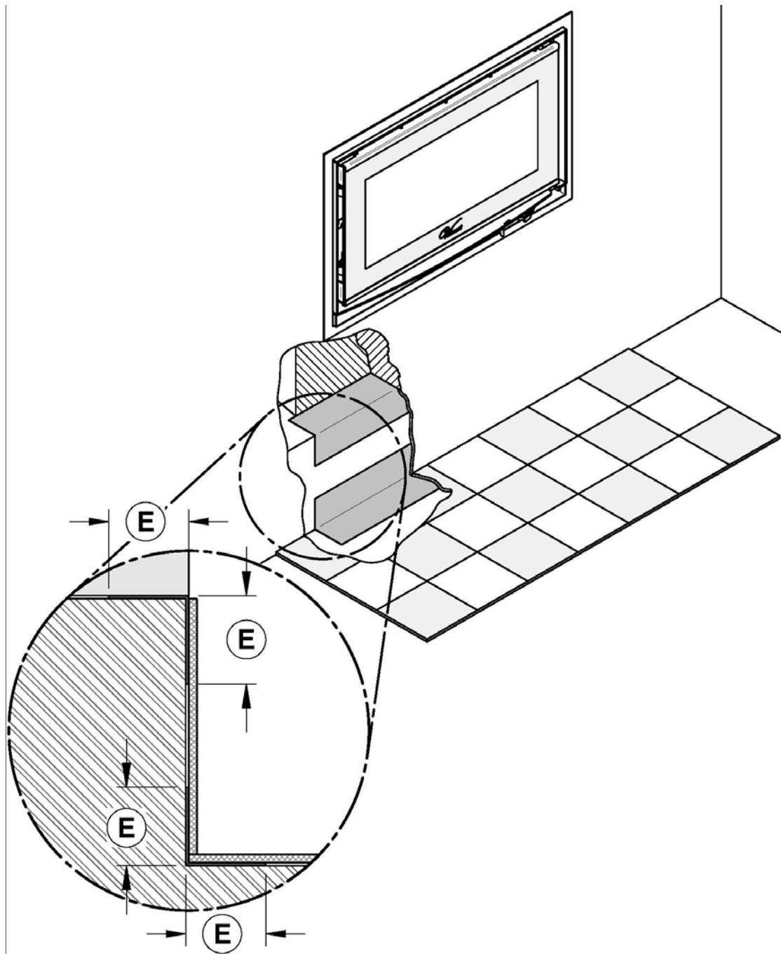
In the case where (F) would be equal to 4", it is suggested that the sheet metal between the base of the fireplace and floor be in one piece.
