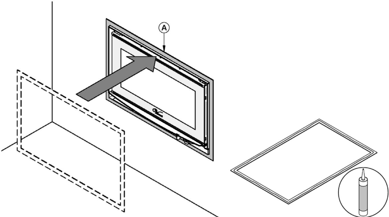
Set the finishing trim around the fireplace frame. If desired, the back of the finishing trim may be glued.
