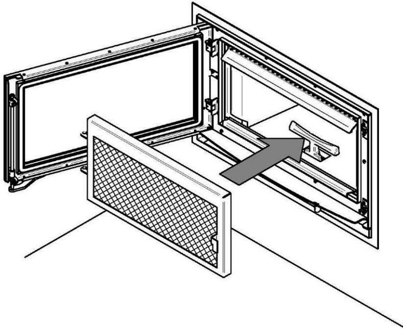
2. Insert the fire screen hinge pins in the holes on the door hinges. Close the fire screen and press firmly against the door opening. Accrocher le pare-étincelle au rivet dans le cadre de porte.
