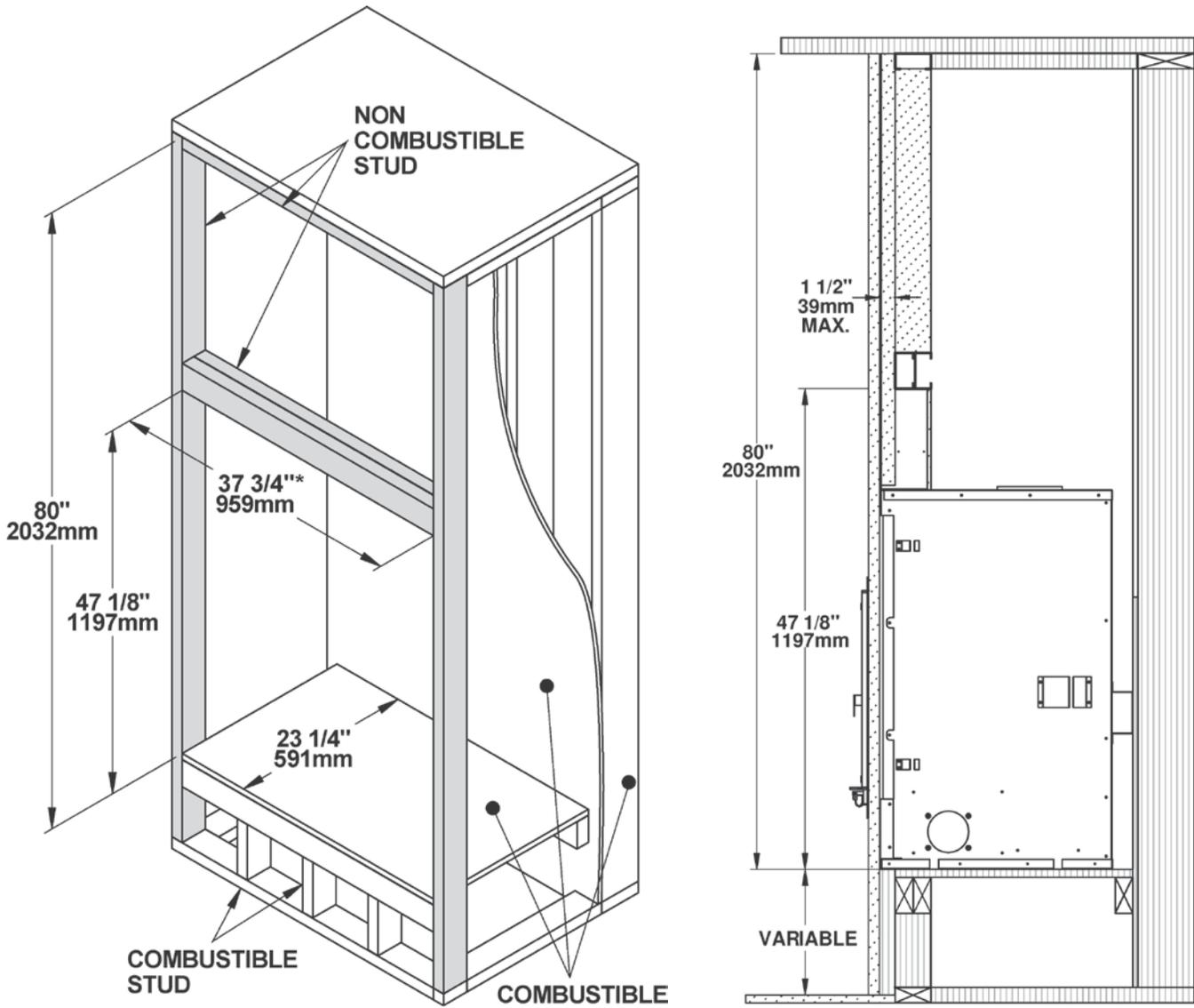
**\* Add 6 "more width to allow installation of the fresh air pipe**
