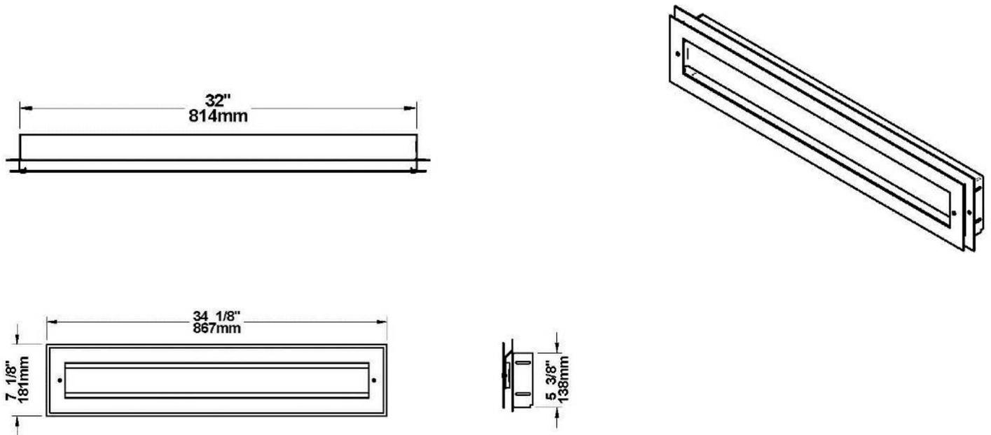
**DIMENSIONS OF ASSEMBLED HEAT DISTRIBUTION BOX AND ADJUSTABLE DECORATIVE PLATE:**
