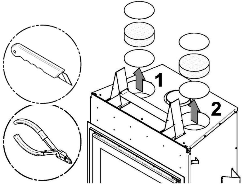
Secure the 6 steel brackets (B) with 6 screws provided (C) on top of the fireplace (3 for each ducting). Insert the ducting (A) (not provided) into each opening and secure it in place using the steel brackets (B) installed previously with 6 other self-tapping screws provided (C).
