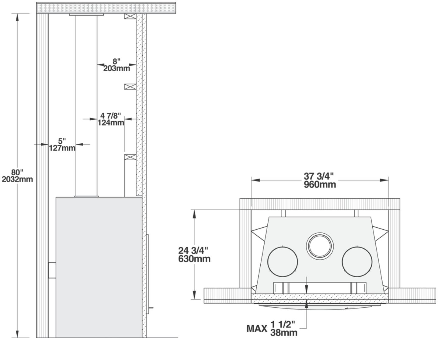
\*When drywall panels or any other finishing material inside the chase around the fireplace is to be used, add its thickness to the measurement.
