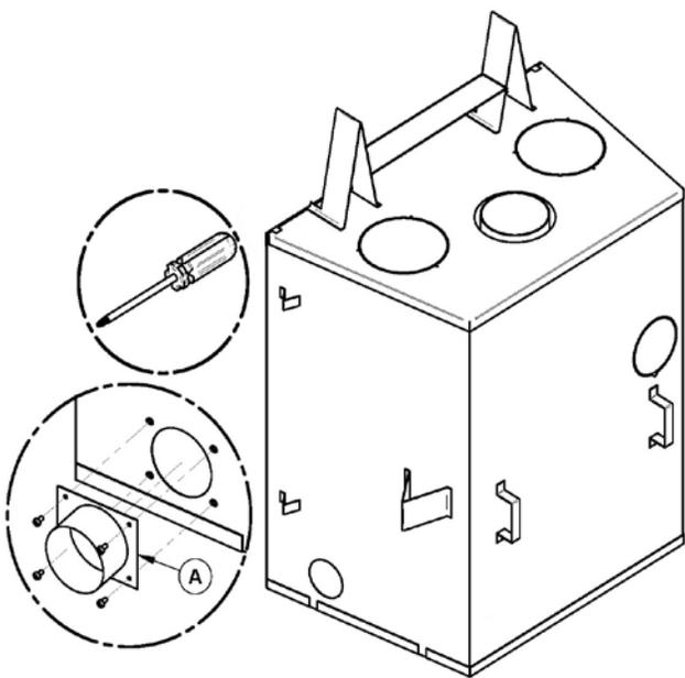
Secure the fresh air intake adapter **(A)** on the fireplace jacket using the 4 screws provided with the kit.
