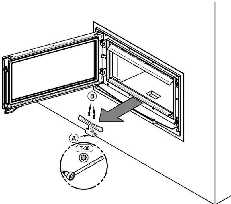
Using a ratchet key and a Torx socket (T-30), unscrew the two Torx screws (B) holding up the andiron (A).
