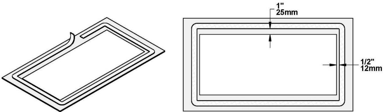
Reinstall the glass, being careful to centre the glass carefully in the door. Do not over-tighten the screws. Note that the two main causes of broken door glass are uneven placement in the door and over-tightening of retaining screws.
