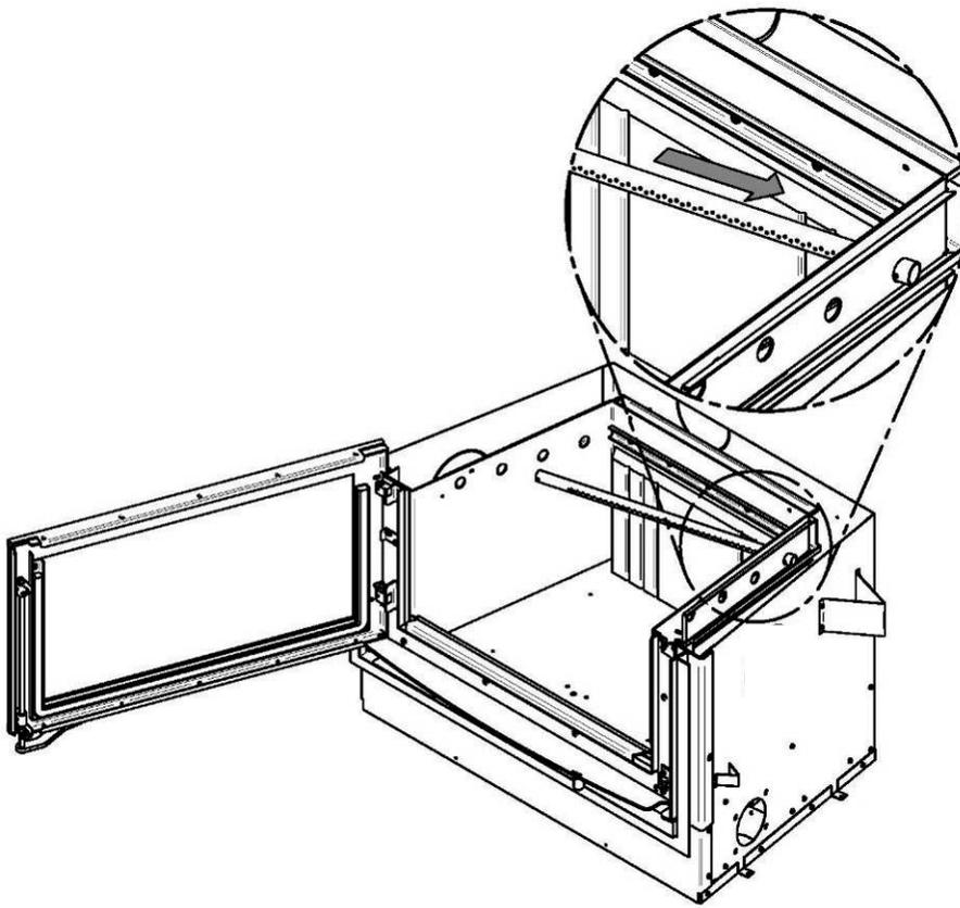
Starting with the rear tube, lean and insert the right end of the secondary air tube into the rear right channel hole. Then, lift and push the tube towards the right inside the hole in the right channel.
