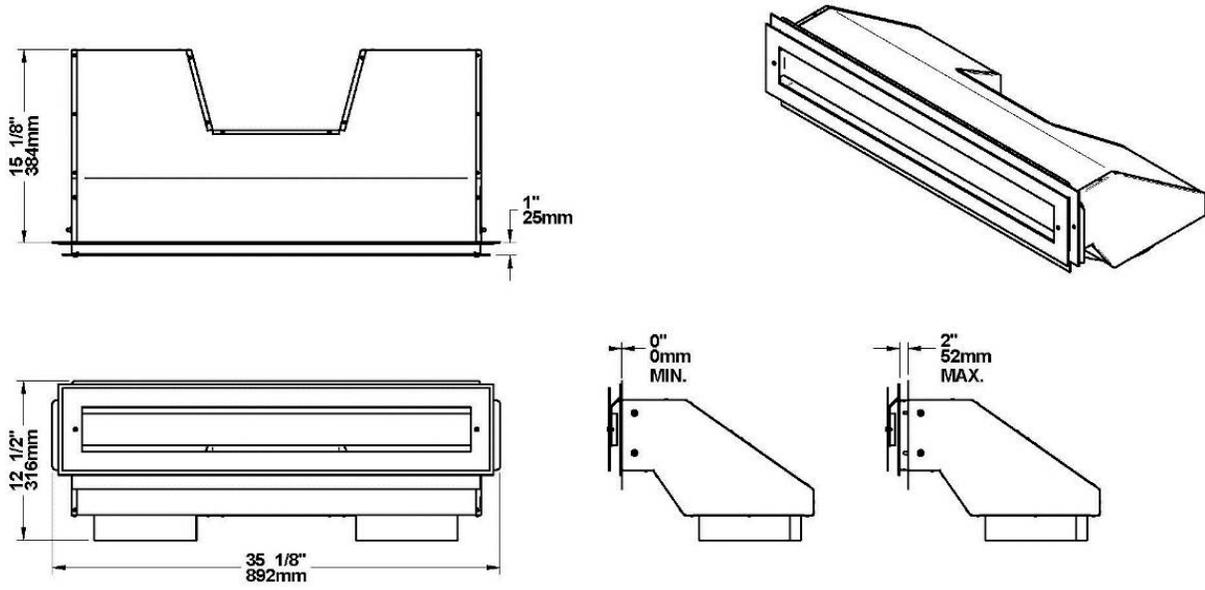
**DIMENSIONS OF TELESCOPING SECTION**
