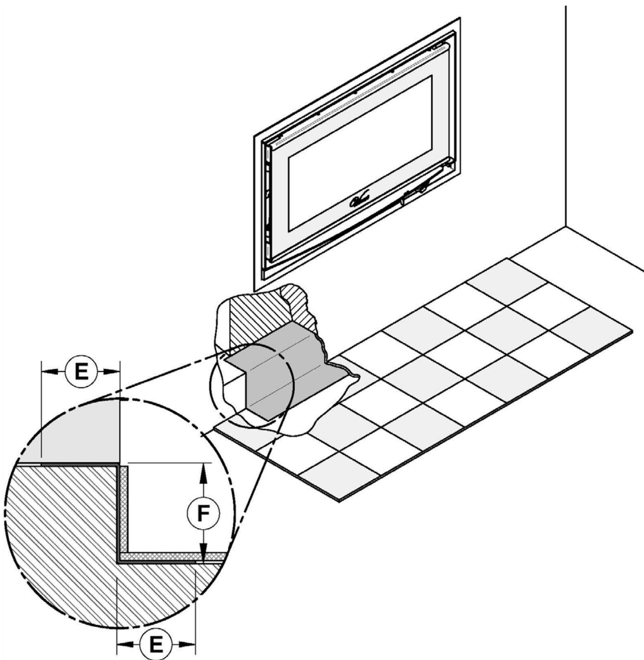
***On the floor or on a raised base of less than 4" installation (R value for the hearth extension required)***
