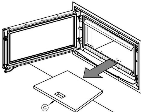
Using a power screwdriver and a 5/16" hexagonal socket, remove the slab holders (D) and the refractory slabs (E) and (F).
