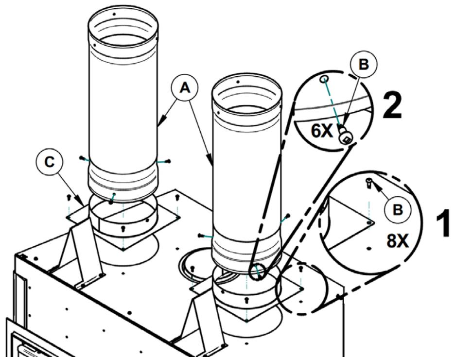
3. Secure the telescoping sections (A) to the heat distribution box (C) with self-tapping screws (B) (3 per telescoping section). Determine the needed height and secure the two parts of the telescoping sections together with 3 self-tapping screws provided. Insert the adjustable frame (D) in the heat distribution box (C), press it against the non-combustible finishing material and secure with 4 screws into the heat distribution box. Set the decorative plate (E) to the adjustable frame (D).
