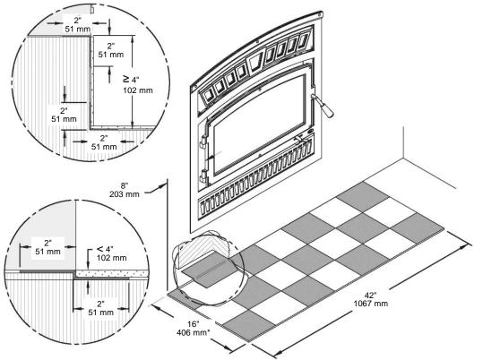
\*If fireplace is installed directly on the floor or on a raised base of less than 4", the hearth extension floor area must extend at least 18" (457 mm) in front of the fireplace with R-value equal to or greater than 1.00. Use 1/2" Micore or refer to manual for equivalent insulation.
