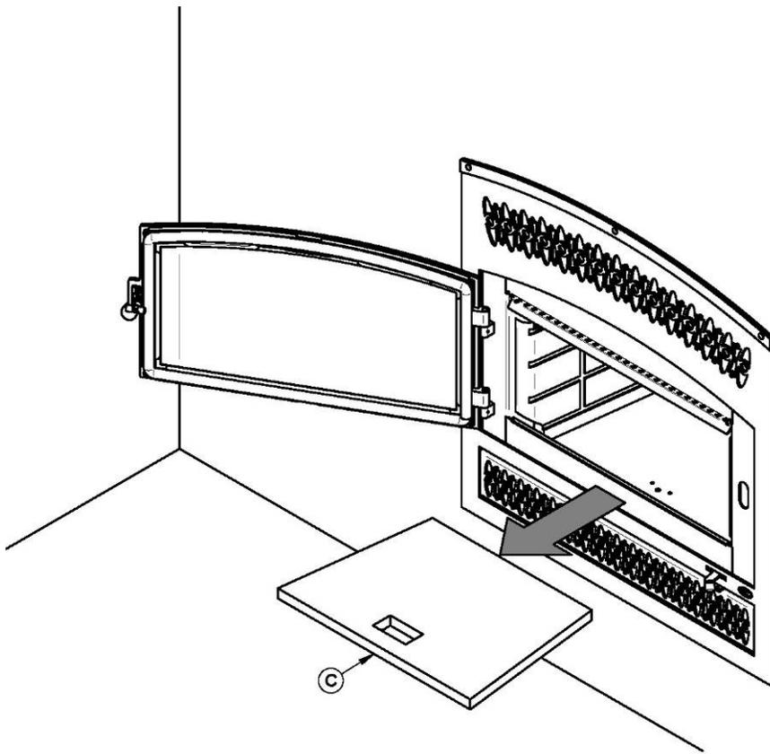
2. Remove the floor refractory slab (C).
