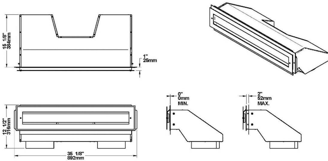
**DIMENSIONS OF TELESCOPING SECTION**
