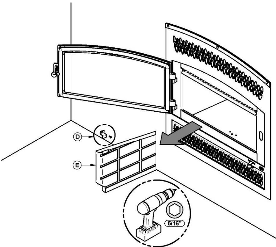
3. Using a power screwdriver and hex tip 5/16", remove the slab holder (D) and the left refractory slab (E).
