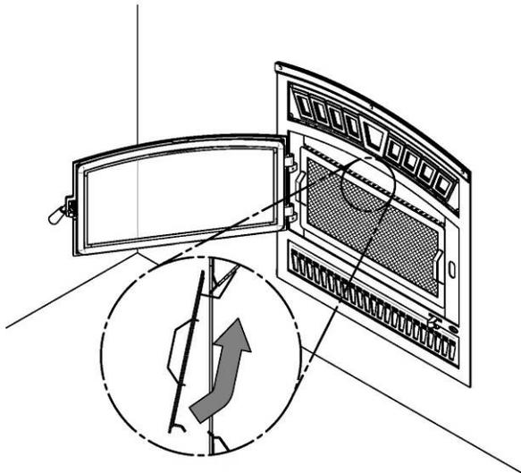
Lean the upper part of the firescreen against the top door opening making sure to insert the top firescreen bracket behind the primary air deflector as in (DETAIL A).
