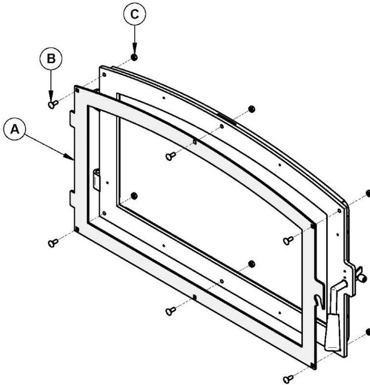
Position the overlay (A) and on the door frame and secure from the inside of the door using the 6 included screws (B) and bolts (C).
