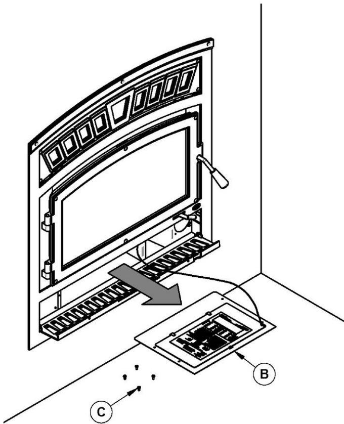
3. Remove and keep the heat shield (B) and the 4 screws (C).
