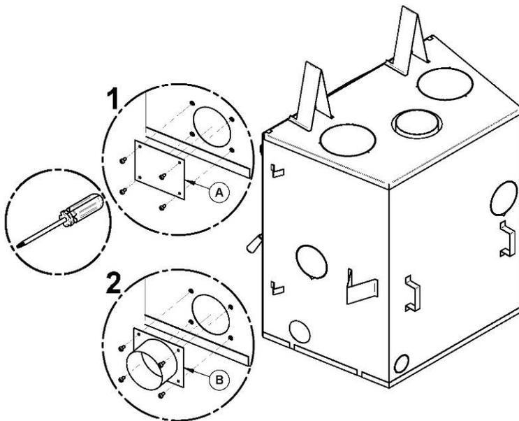
(1) Using a Philips screwdriver, remove the four screws holding the rectangular plate **(A)** on the right of the fireplace jacket. If the location 2 or 3 has been chosen, use pliers to remove the knock-out.
