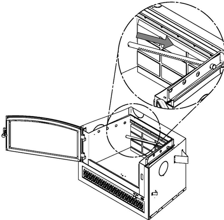
4. Starting with the rear tube, lean and insert the right end of the secondary air tube into the rear right channel hole. Then, lift and push the tube towards the right inside the hole in the right channel.
