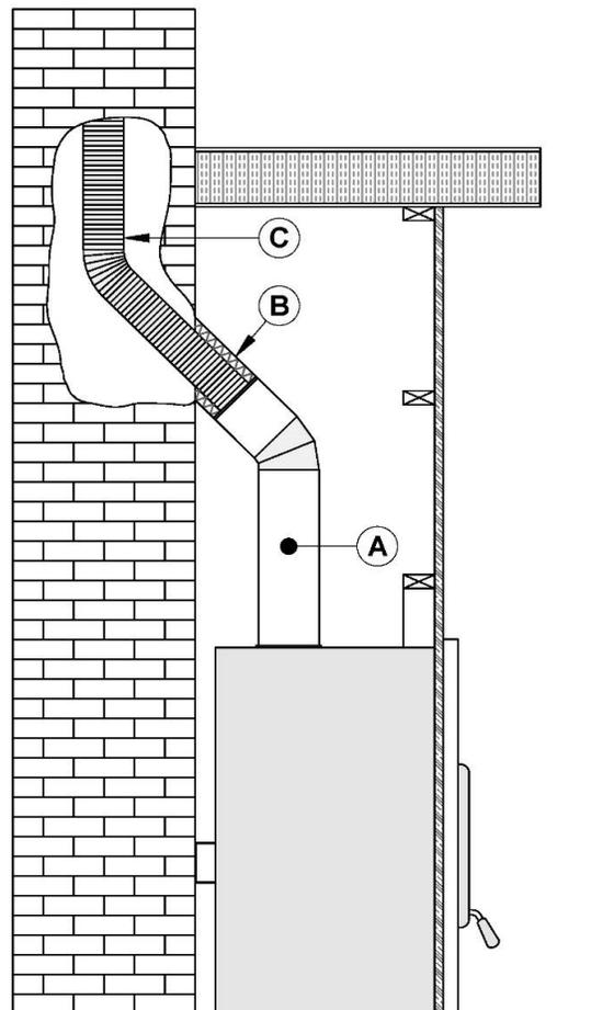
**Note:** Make sure the liner exceeds at least 12" (30 cm) the top of masonry chimney.
