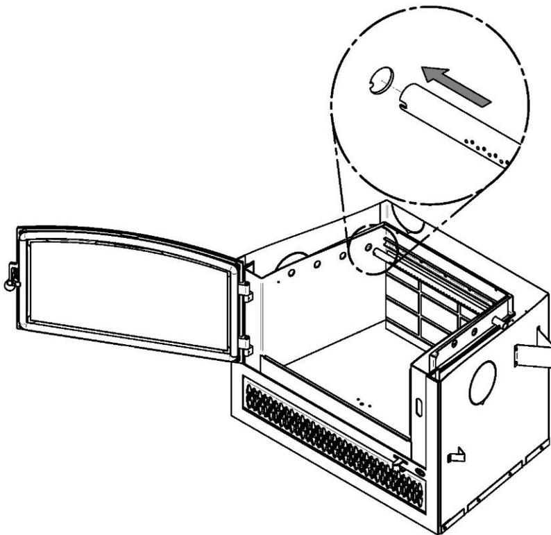
5. Align the notch in the left end of the tube with the tab of the left air channel hole.
