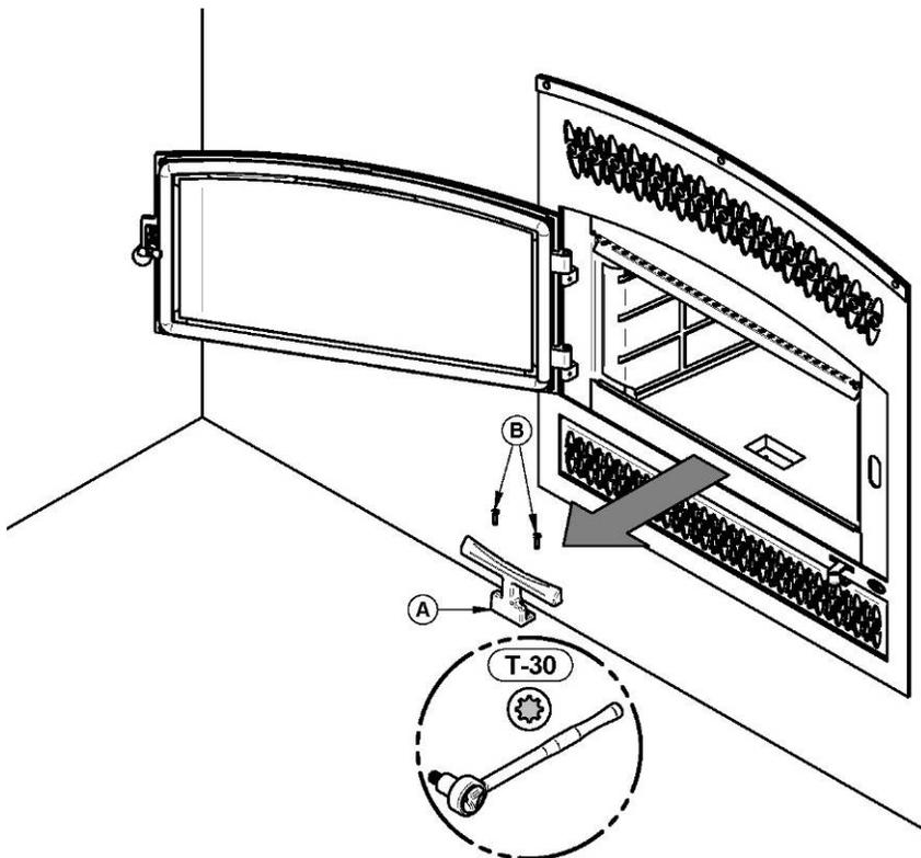
1. Using a ratchet key and a Torx (T-30), unscrew the two Torx screws (B) holding up the andiron (A).
