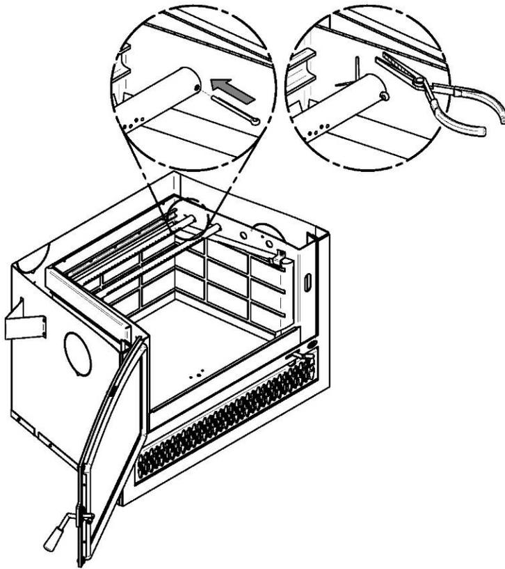
6. Insert a cotter pin in the last hole on the right side of the tube. Then bend the tabs on the pin to keep in place.
