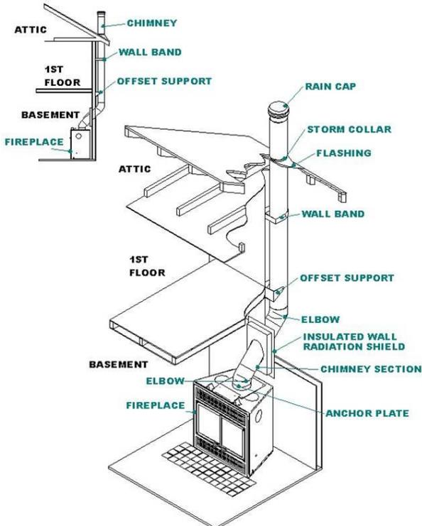
Figure #13: Isolated Chase Chimney Installation
