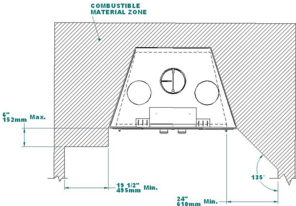
Figure #15: Chimney Enclosure
