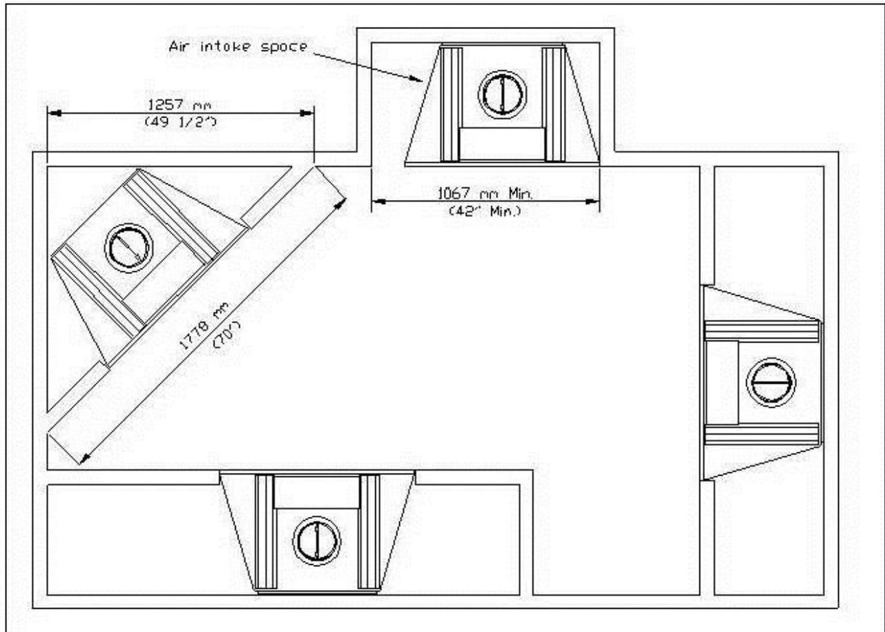
Figure #3: Possible Chimney Configurations
