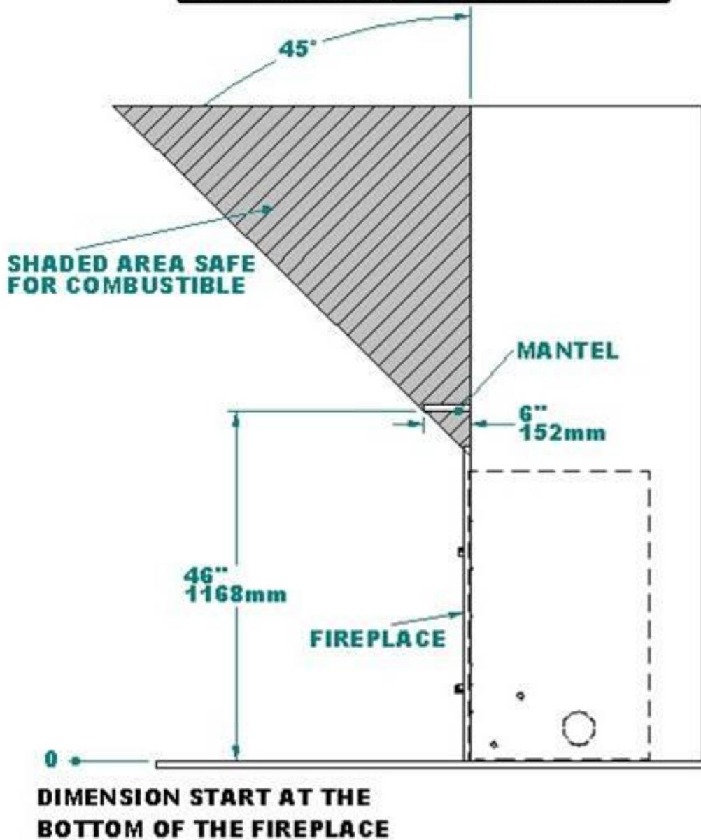
Figure 16b : Combustible material positioning
