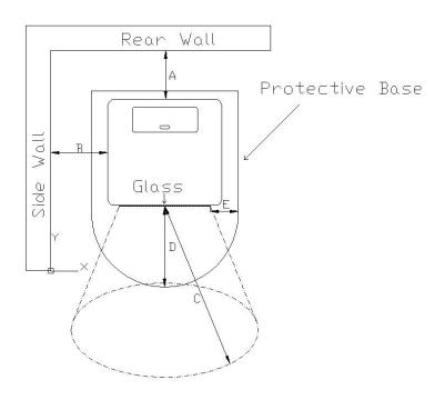
While installing the stove, the fire regulations and chimney's instructions must be complied. For any related questions please ask the chimney installer. Minimum distances to be observed in flammable or heat-sensitive materials (eg furniture, wallpaper, wood panels) (see diagram below) are:
