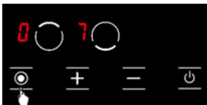
Cooking level is displayed by itself without a point ( • ) icon when a single hob of the double heater is activated by touching the special function selection key. (See Fig. 25)
