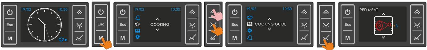
2. Using the **▲** or **✕** buttons (or by rotating the Function Selector Button), you may scroll through all available food types. Press **✓** when the desired food type is on the screen.
