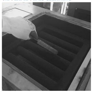
Remove the metal plate on the product's upper table and brush the exchanger pipes with the brush provided with the stove or boiler. Do this once a week.
