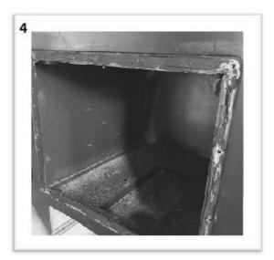
After cleaning, the oven section and then the oven door must be reinserted. Heat-resistant silicone should be used in the oven frame when installing the compartment screws.
