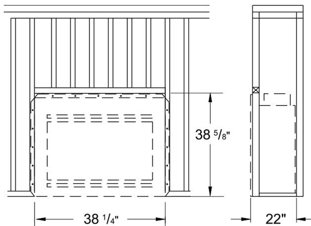
**Figure 1 - Framing Dimensions**
