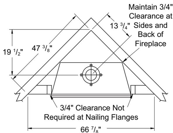
**Figure 2 - Corner Installation**
