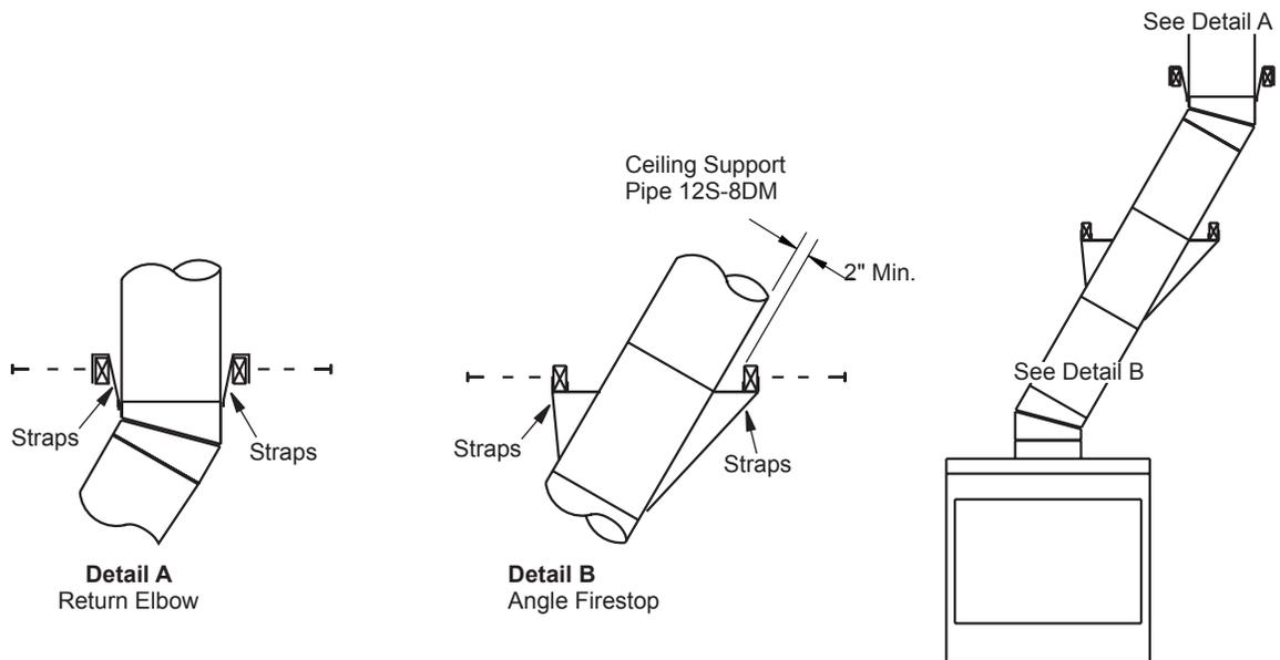
**Figure 10 - Ceiling Support Pipe 12S-8DM**
