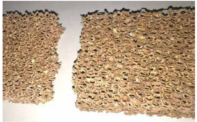
Combustor Problem - Broken Combustor
