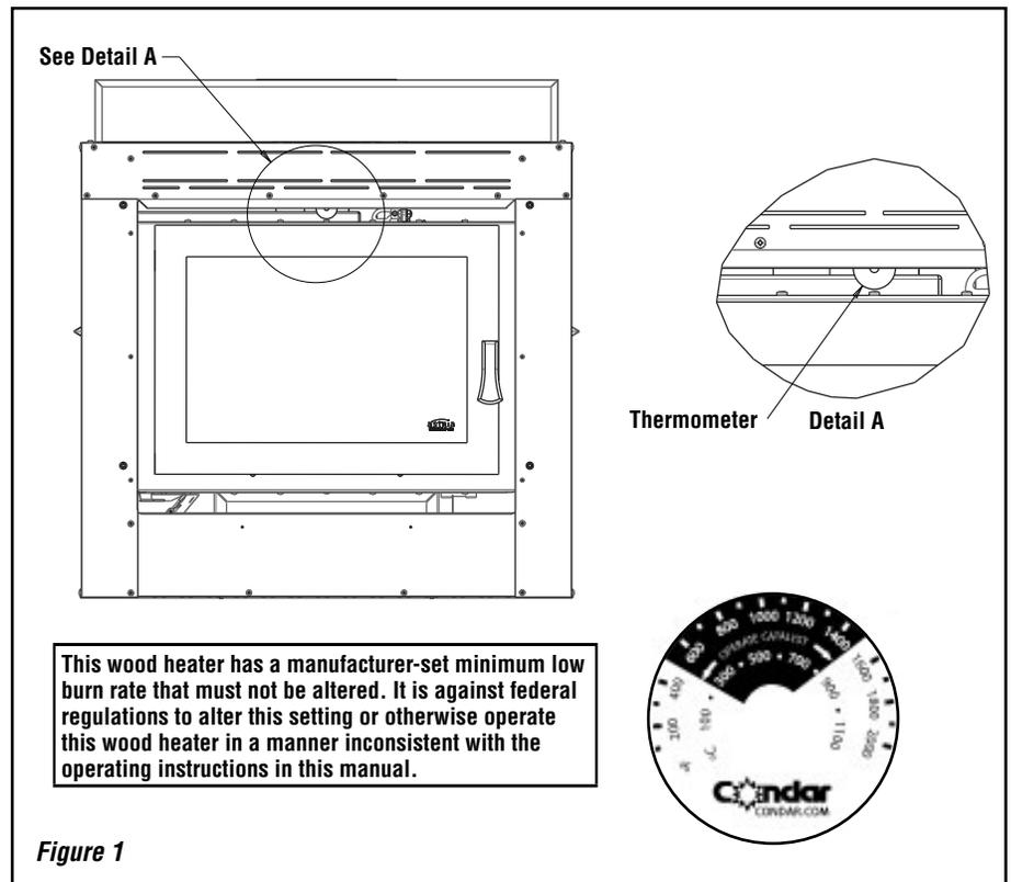
This manual describes the installation and operation of the IHP model WRT3920WS catalytic equipped wood heater. This heater meets the 2020 U.S. Environmental Protection Agency's certified to comply with 2020 particulate emission standards using crib wood. Under specific test conditions this heater has been shown to deliver heat at rates ranging from 10,900 to 35,600 Btu/hr.
