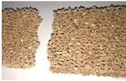
**Combustor Problem - Broken Combustor**
