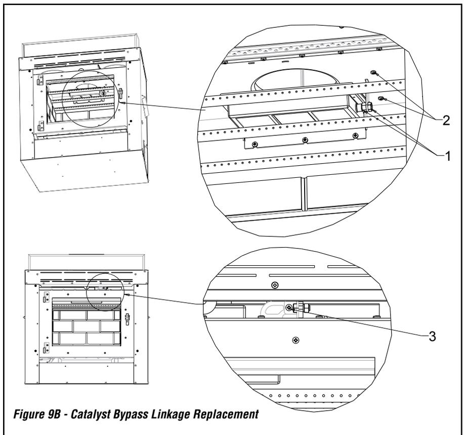
Figure 9B - Catalyst Bypass Linkage Replacement
