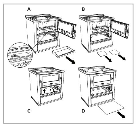
Picture 31 - Fume-circuit inspection.
