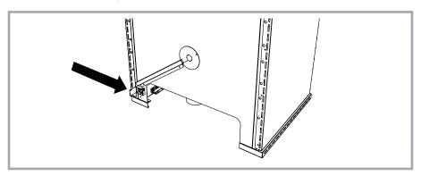
Picture 16 - Position of the terminal board for the connection to the network
