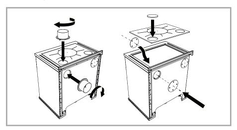
Picture 7 - Multiflue cooker, predisposition of the correct flue outlet
