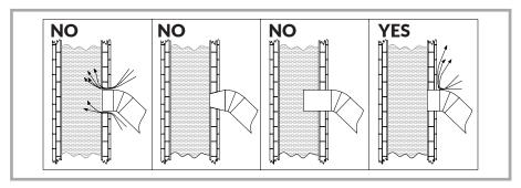
Picture 9 - Examples of correct and incorrect connection of the chimney
