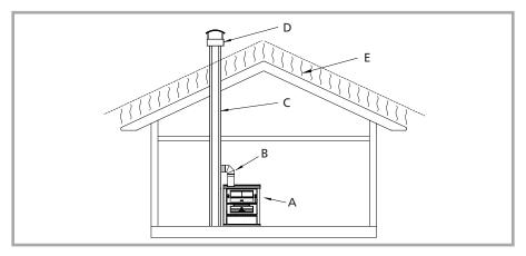
Picture 4 - Components of the chimney, A= cooker, B= conjunction, C= flue, D= chimney, E= reflow zone
