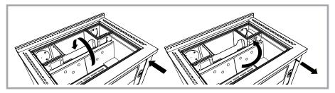
Picture 19 - Starting key. With lever outside, the key is open and the starting is easier; with lever inside the key is closed for the normal working
