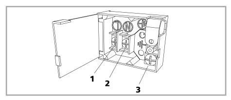
Picture 17 - Terminal board for the connection to the network: 1. Line 2. Neutral 3. Earth.
