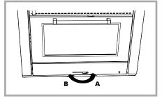
Picture 24 - The valve is open in correspondence of the position marked by letter "A", while is closed in the position marked with letter "B" (ML Range).
