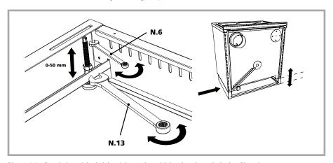
Picture 14 - Regulation of the height of the cooker with hex key through the levelling pins.
