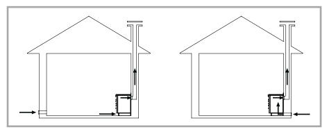
Picture 11 - Installation with air intake in the room of installation and installation with air intake directly connected to the wood fired cooker.
