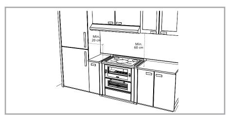
Picture 3 - Minimum safety distances when using suited spacers for the installation into furniture
