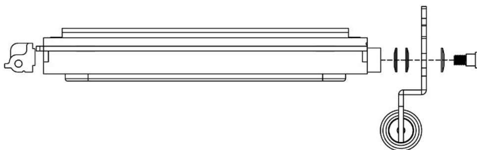
Picture 33 – Correct position of the rounded washers.
