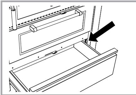
Picture 26 - Switch to light the oven (M - MZ range).
