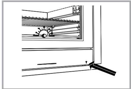
Picture 27 - Switch to light the oven (ML range).
