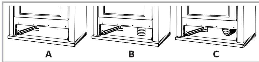
Picture 12 - Possible connections of the air intake of the cooker. A = External air intake not connected B = External air intake on the floor C = External air intake on the wall.
