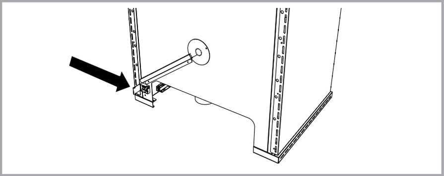
Picture 16 - Position of the terminal board for the connection to the network
