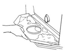
screwdriver to scrape away and loosen any remaining debris. Continue this process until all remaining ash debris is removed and all of the air holes in the burn pot are clear.
