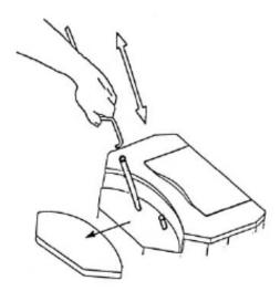
Cleaning is accomplished by pulling up and pushing the two exchanger scraper rods that protrude out of of the stove. These rods can be found on the very the stove underneath the colored accent panel. are two holes in the accent panel where the rods Due to the placement of these two holes, removal of the colored accent panel is not necessary cleaning.
