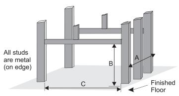
Note: All studs on top and sides of unit must be on edge.
