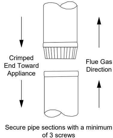
Figure 15.3 - Chimney Connector (Appliance Pipe)
