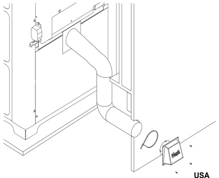
Figure 16.2 - Floor Installation
