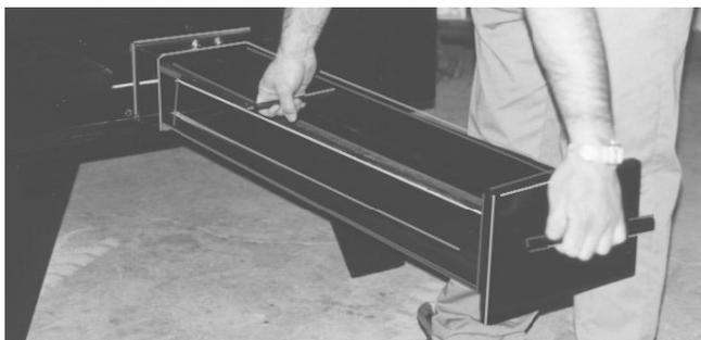
1. The ash tray must be checked weekly and emptied as necessary. Ensure that the ash tray is securely closed after each cleaning.
