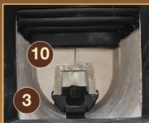
Fire head is surrounded by molded, refractory cement.
