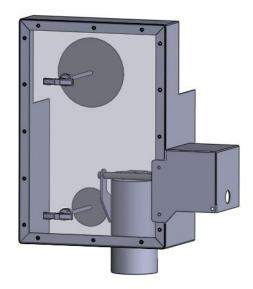
Top Lever: Primary Air Adjust Bottom Lever: Secondary Air Adjust
