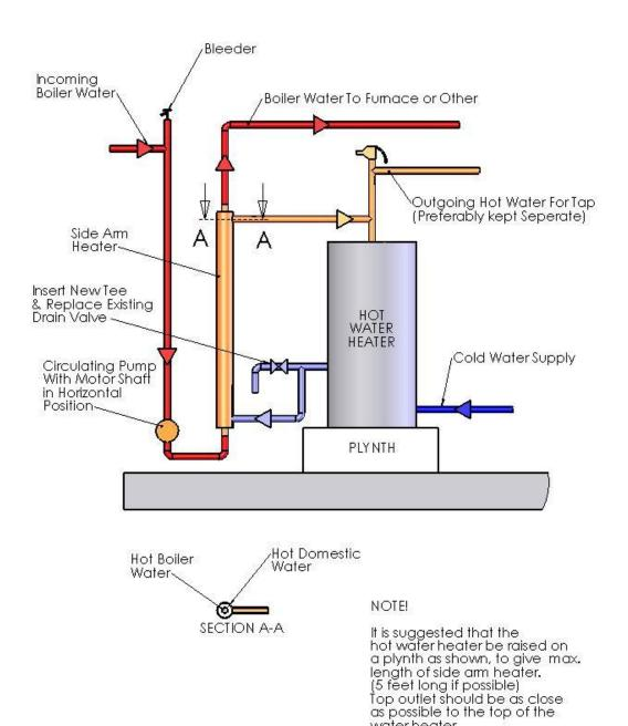
SCHEMATIC #4 - CONNECTING SIDE ARM HEATER TO DOMESTIC WATER TANK
