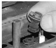
Pilot Cap Clip Diagram 3
