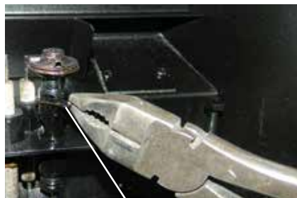
Pilot Cap Clip Diagram 3
