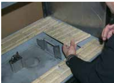
Remove Left & Right Side Base Brick Panels
