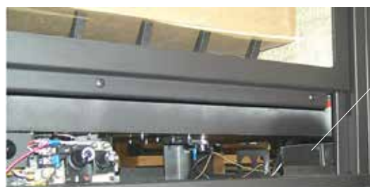
Remove cover to access Terminal Block
