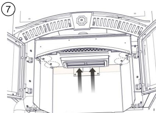
Reach in through the opening of the bypass door to access fasteners.
