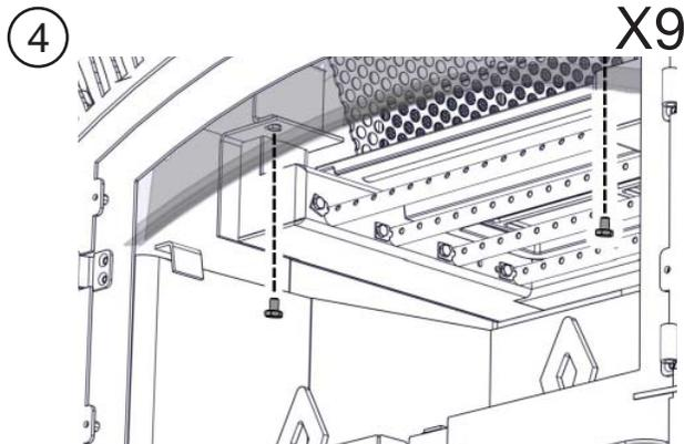
Remove front two nuts and bolts as shown.
