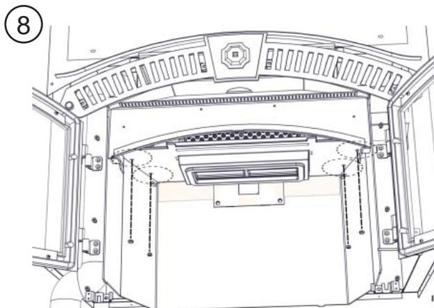
Remove nuts & bolts on either side of appliance while supporting the baffle.
