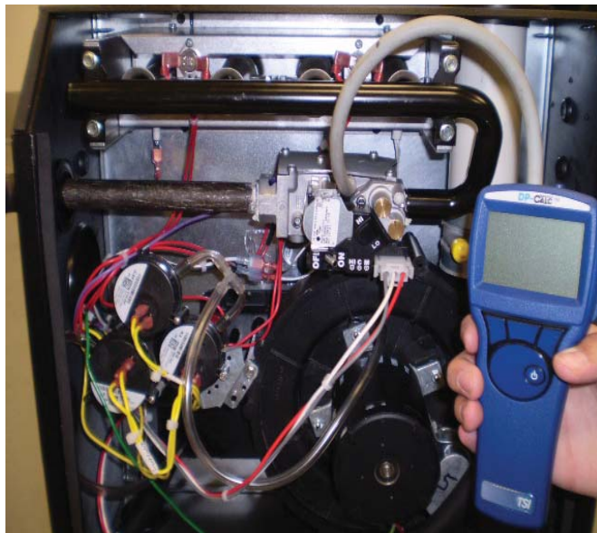
FIGURE 30 - MANOMETER MEASURING GAS MANIFOLD PRESSURE
