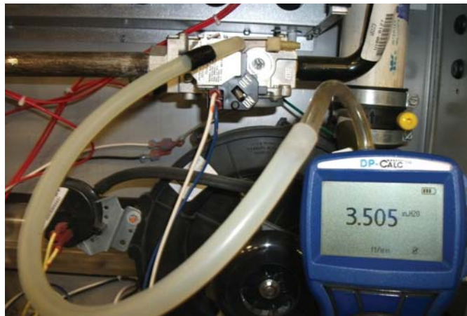
FIGURE 30 - MANOMETER MEASURING GAS MANIFOLD PRESSURE
