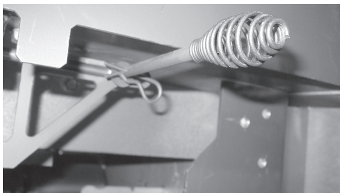
Figure 4.36 Reinstalling Hairpin Clip and Washer
