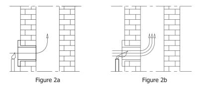
If air flow in the chimney is weak (Fig. 2a), check accuracy of chimney. Chimney should be located within interior of an object, and if it's on external walls of an object, it is recommended to insulate the chimney.
