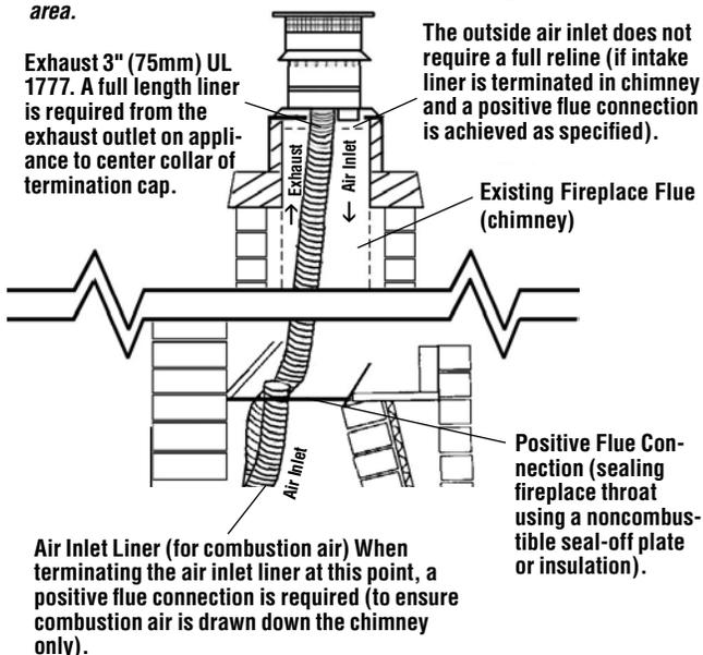
**Figure 6a - Terminating Air Inlet in Chimney**
